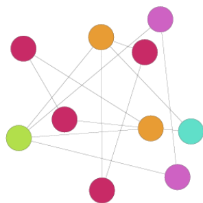
FIG. 5.1: A bidirectional 10-node network. Nodes that are the same color represent a symmetry cluster, and links (gray lines) represent the network connectivity.
