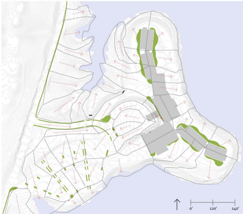
Figure 25. Designed Bioretention Cells Map
