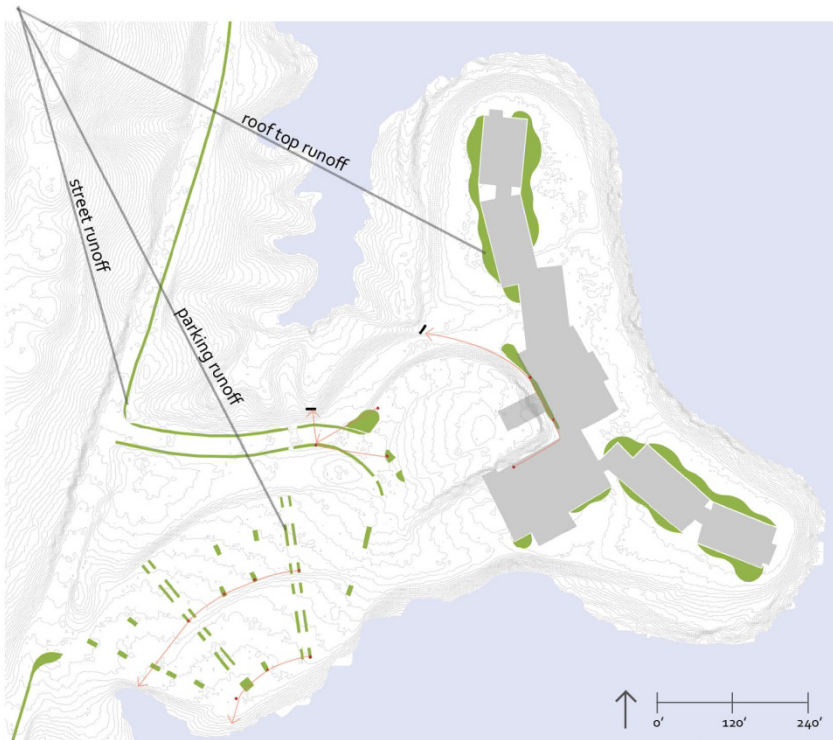
Figure 25. Designed Bioretention Cells Map
