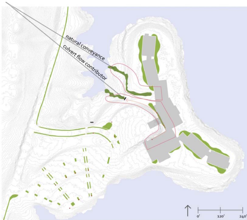
Figure 27. Designed Bioswales Map
