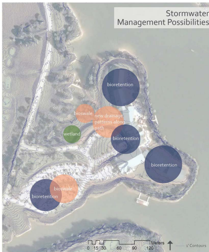
Figure 21. Stormwater Management Possibilities Map
