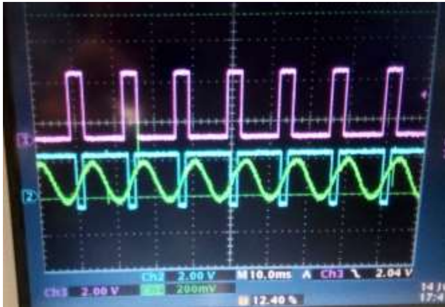
Figure 55. Position, PLL, and Ignition Signals from the Z Elimination Code on the Oscilloscope
