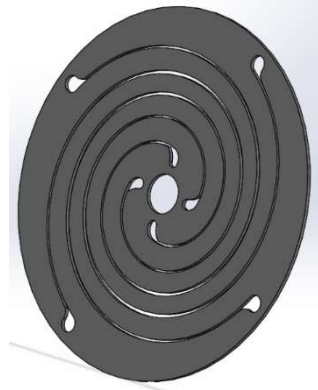
Figure 2. Flexure bearing used in OLEA system
