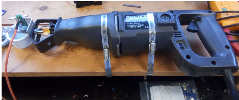
Figure 49. Reciprocating Saw as a Test Bench
