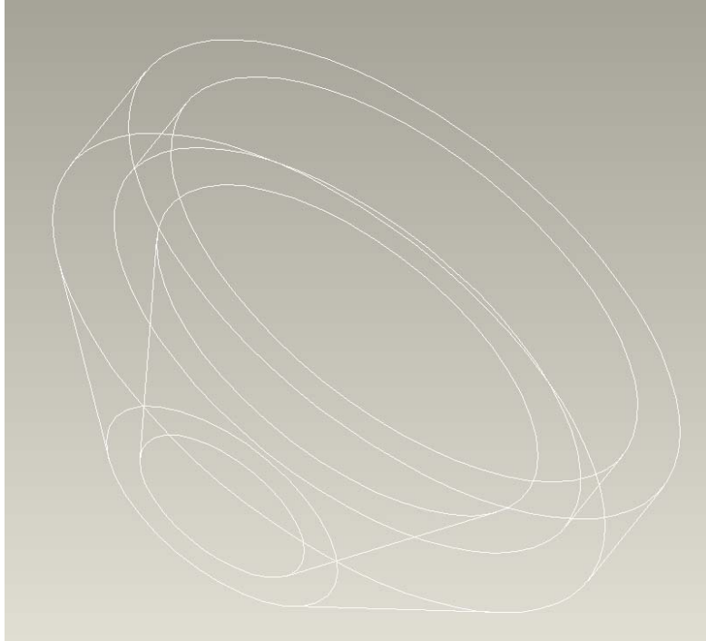
Figure 3.25: CAD Drawing of a Straight Cap (Drawing Courtesy of Mr. Travis Michalak of the AFRL)
