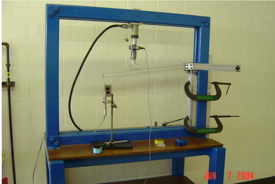
Figure 3.13: Picture Taken at Maximum Applied Load on an 80/20 Corner Joint
