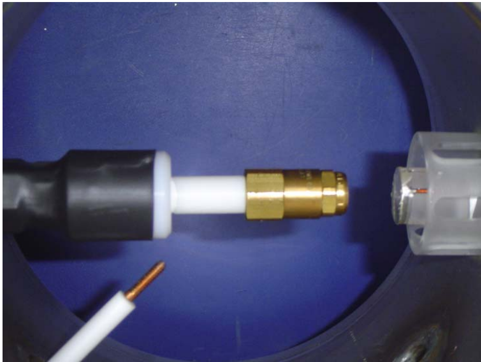
Figure 3.20: Nozzle Plumbing Position Approximately 13 mm from Heated Surface
