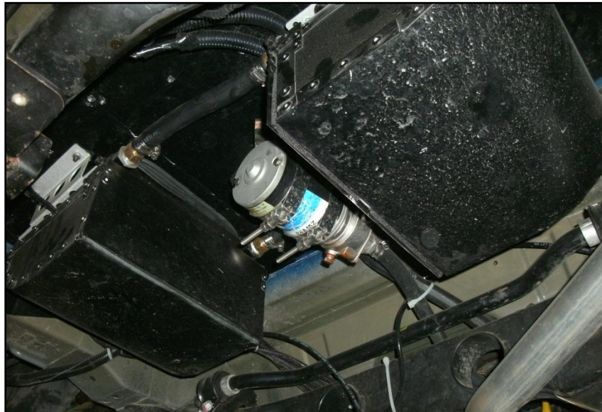
Figure 50. Heat Exchangers with Dampers Installed
