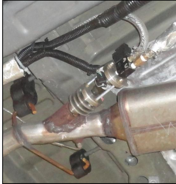
Figure 56. Urea Injection System
