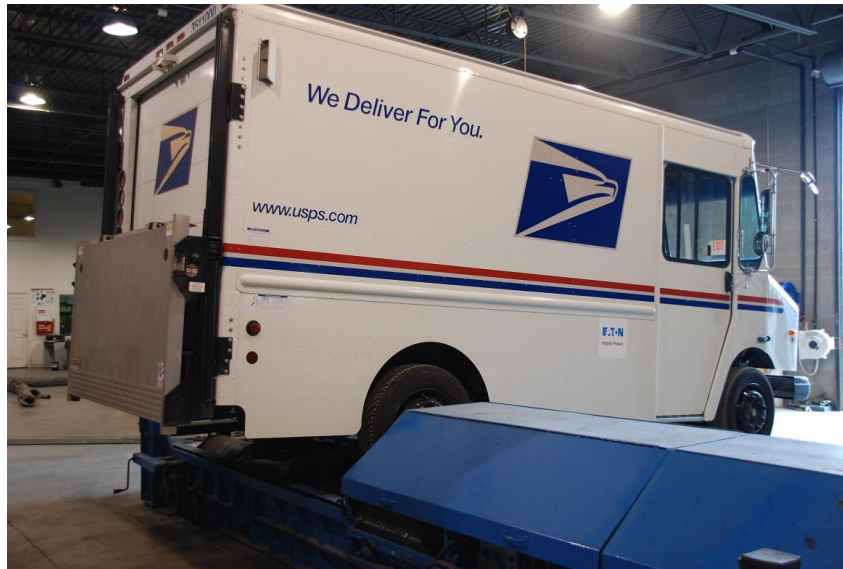
Figure 1. WVU's medium duty chassis dynamometer with a Hybrid USPS Step Van installed at WVU's Westover Laboratory
