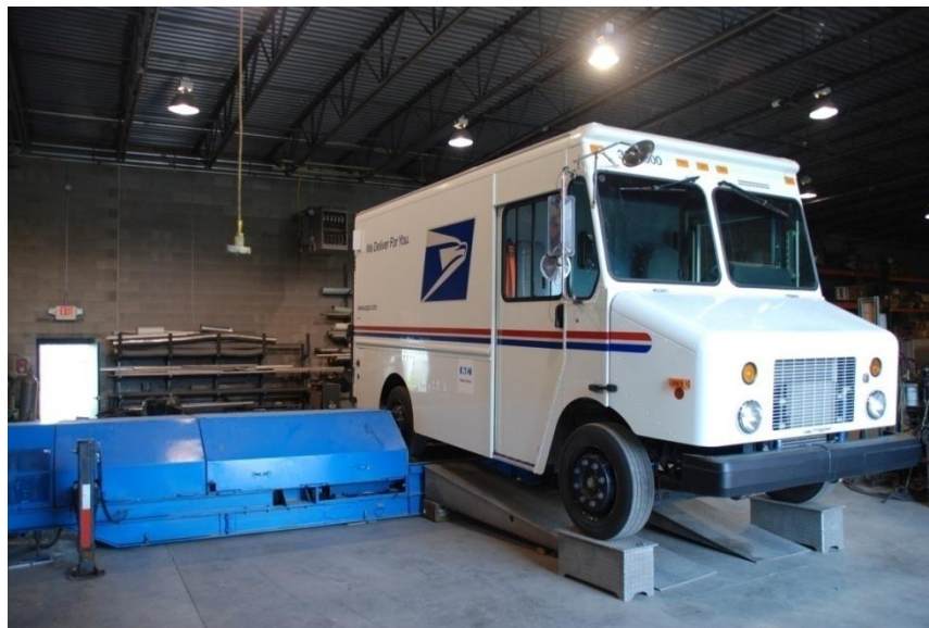
Figure 3. One of the two USPS step van step employed on the chassis dynamometer
