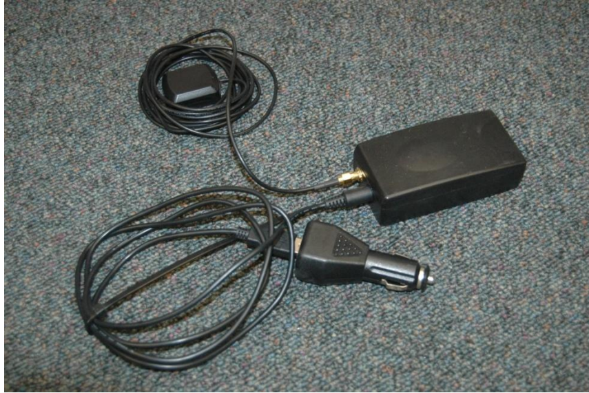
Figure 7. GPS unit used for the on road coastdowns
