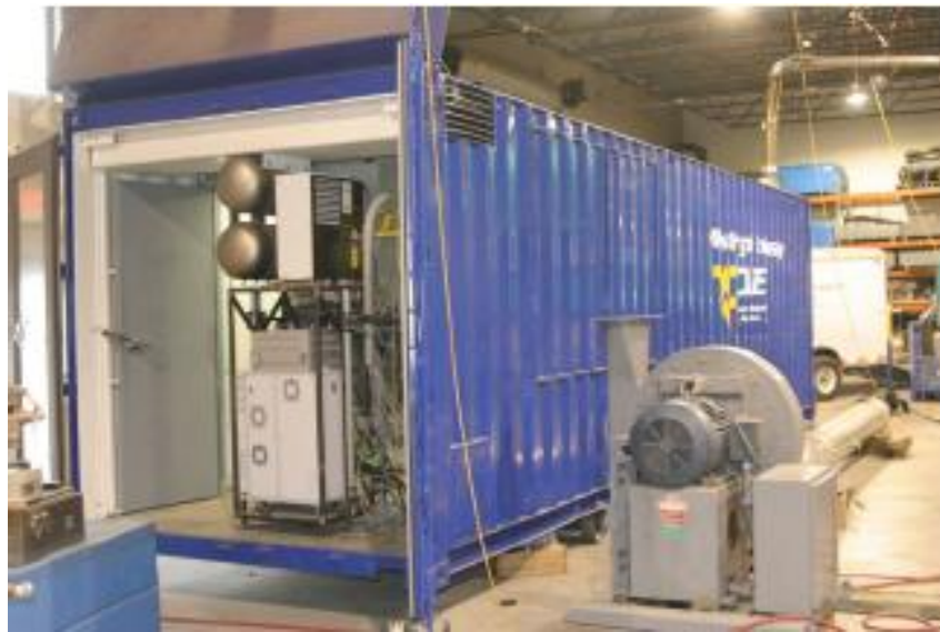
Figure 2. WVU's 2007 analytical trailer utilizing EPA 40 CFR Part 1065 regulation at WVU's Westover Laboratory
