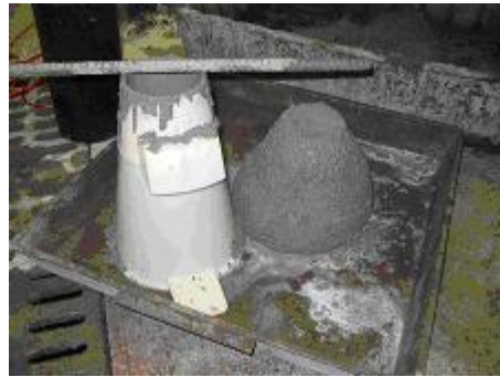
Figure 5.3: Slump of CFLMC (5")
