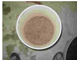
Figure 3.1 e: Fine aggregate (sand)
