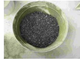
Figure 3.1 c: Coarse aggregate (#8)
