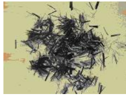
Figure 3.1 b: Carbon Fibers (0.5 in.)
