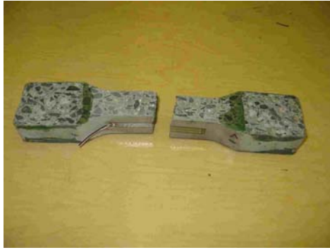
Figure 4.9: Fractured Tensile Specimen
