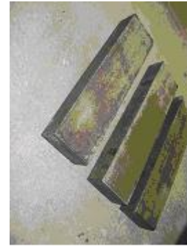
Figure 4.14 (f): Cured flexure specimen
