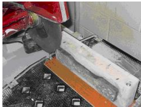
Figure 4.5: Saw cutting top 0.5" off specimen
