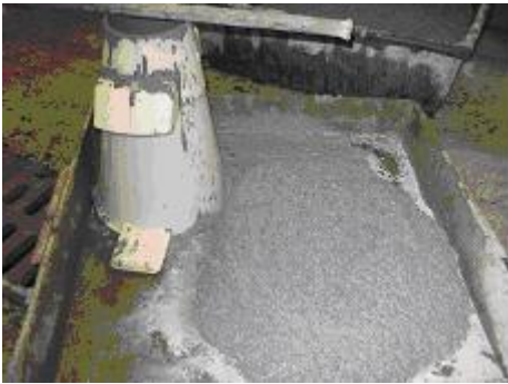
Figure 5.2: Slump of LMC (8")
