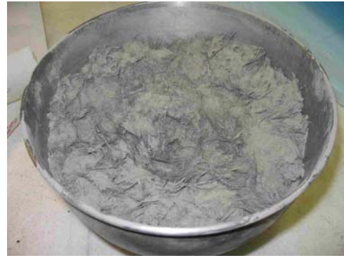
Figure 3.6: Cement and Carbon Fibers
