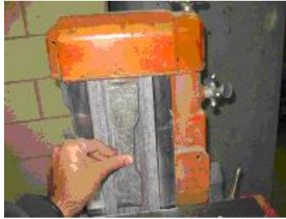
Figure 4.6: Sanding of specimens
