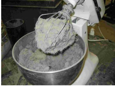
Figure 3.5: Dry mixing of carbon fibers with cement
