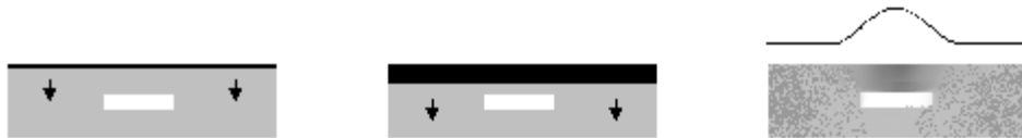
Figure 3.3.1 Heat flow due to a flash pulse. Initially the pulse causes thin layer of uniform heat on the surface (Left). Heat flows into the sample (Center). When a defect is encountered, the heat is trapped between the defect and the sample surface, giving rise to lateral heat flow above the defect (Shepard et al. 1999).
