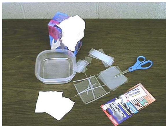
Figure 4.5.2. The delamination prepared by enclosing an air pocket between two polypropylene sheets.
