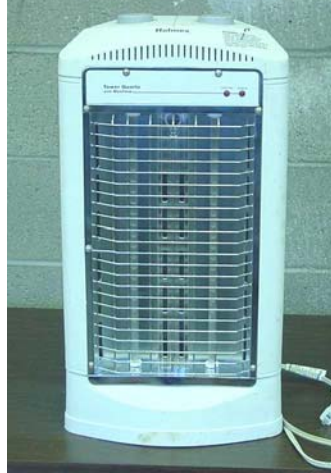
Figure 4.4.1. The quartz tower heater used for heating the specimens in the laboratory.
