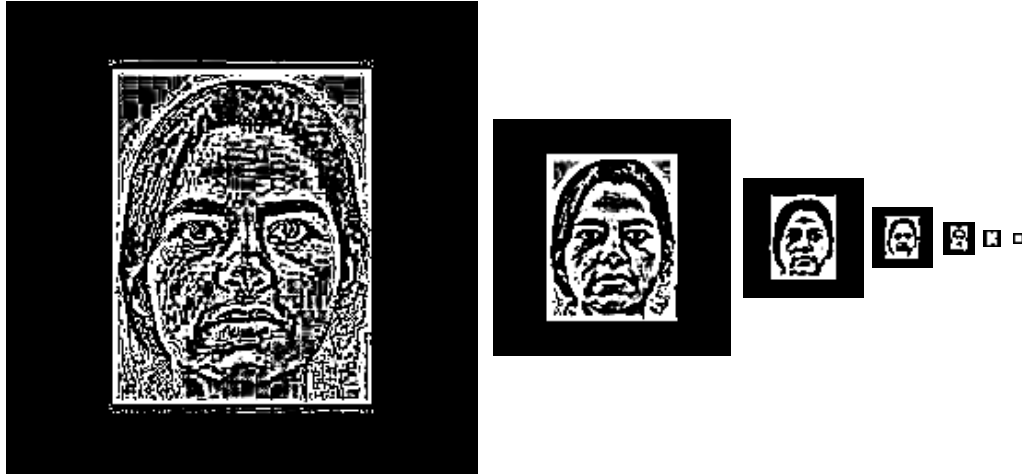
Figure 4.5: The Laplacian pyramid of a frontal image from Level 0 to Level 6.
