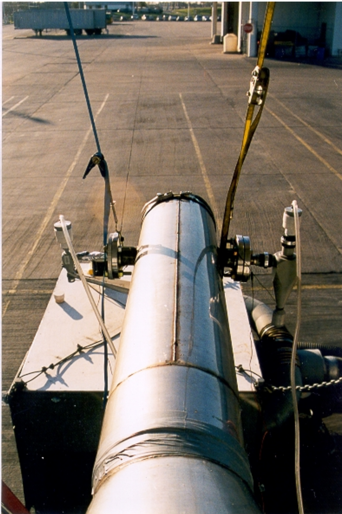
Figure 3.4 – Cyclones and Dilution Tunnel Extension in Use During DART Testing
