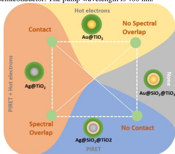
Figure 5.14. The variables that control the possible plasmonic enhancement mechanisms for extending photoconversion. Connecting the line between the properties of the given core@shell nanoparticle gives the corresponding enhancement mechanisms present.
