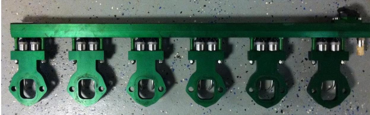
**Figure 26 - CNG Injection Rail**
