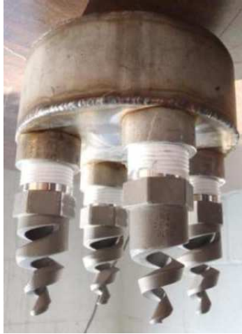
Figure 5.6: Stainless Steel Nozzles attached to Liquor Distributor
