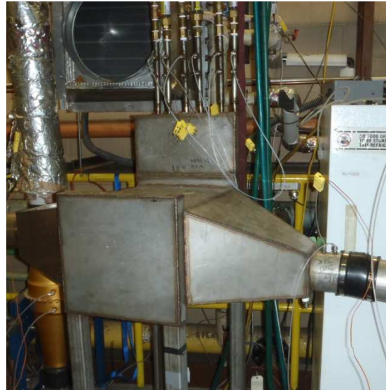
Figure 4.4: Heat Exchanger Housing
