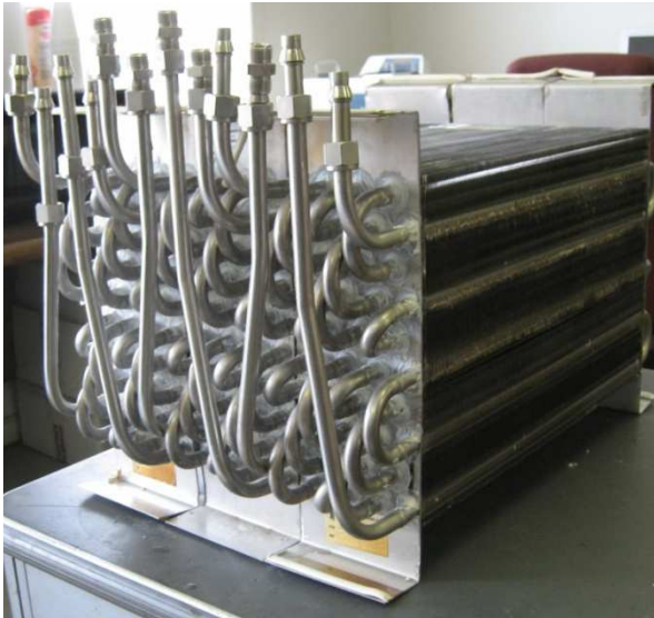
Figure 4.3: Three Heat Exchanger Units
