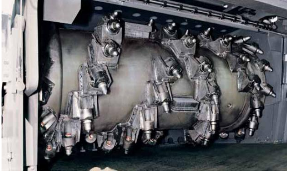
Figure 1-5 Rotating Drum and Carbide-Tipped Cutting Tools (Wirtgen, 2010)
