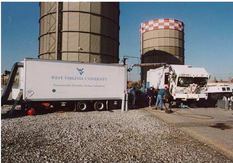
Figure 4.1 A historical photograph showing one of the WVU Transportable Laboratories testing a New York city Department of Sanitation truck at Brooklyn Union Gas site.
