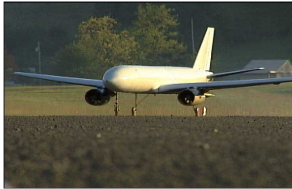
Figure 6.2.2 High visibility paint scheme
