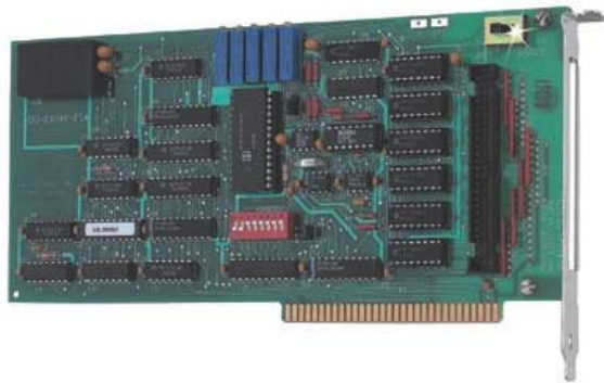
Figure 3.5.5 CIO-DAS48-PGL data acquisition card
