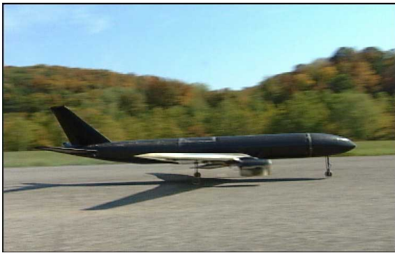
Figure 6.1.5 High speed taxi test
