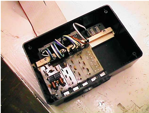
Figure 3.5.8 Signal conditioning interface
