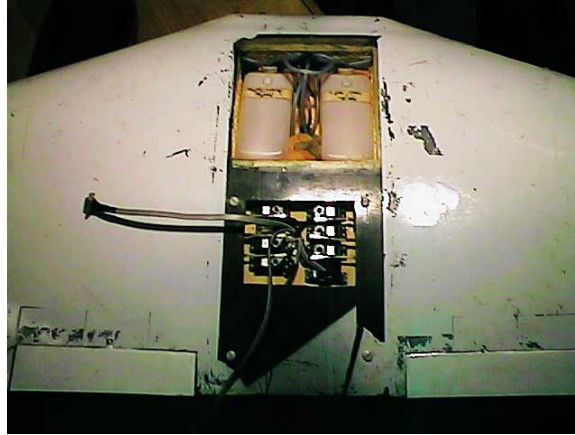
Figure 3.2.5 Wing servo system and fuel bay
