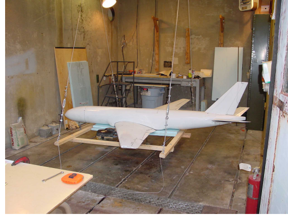
Figure 3.6.2 Pendulum setup (axis-Iy)
