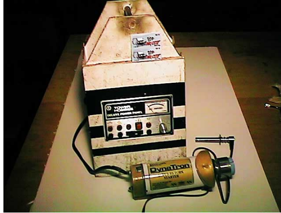
Figure 3.4.2 Field box starting equipment for propulsion system
