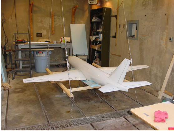
Figure 3.6.1 Pendulum setup (axis-Ix)
