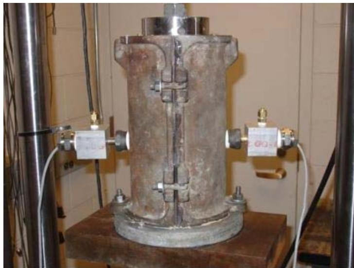
Figure 2.6 Formwork measuring device
