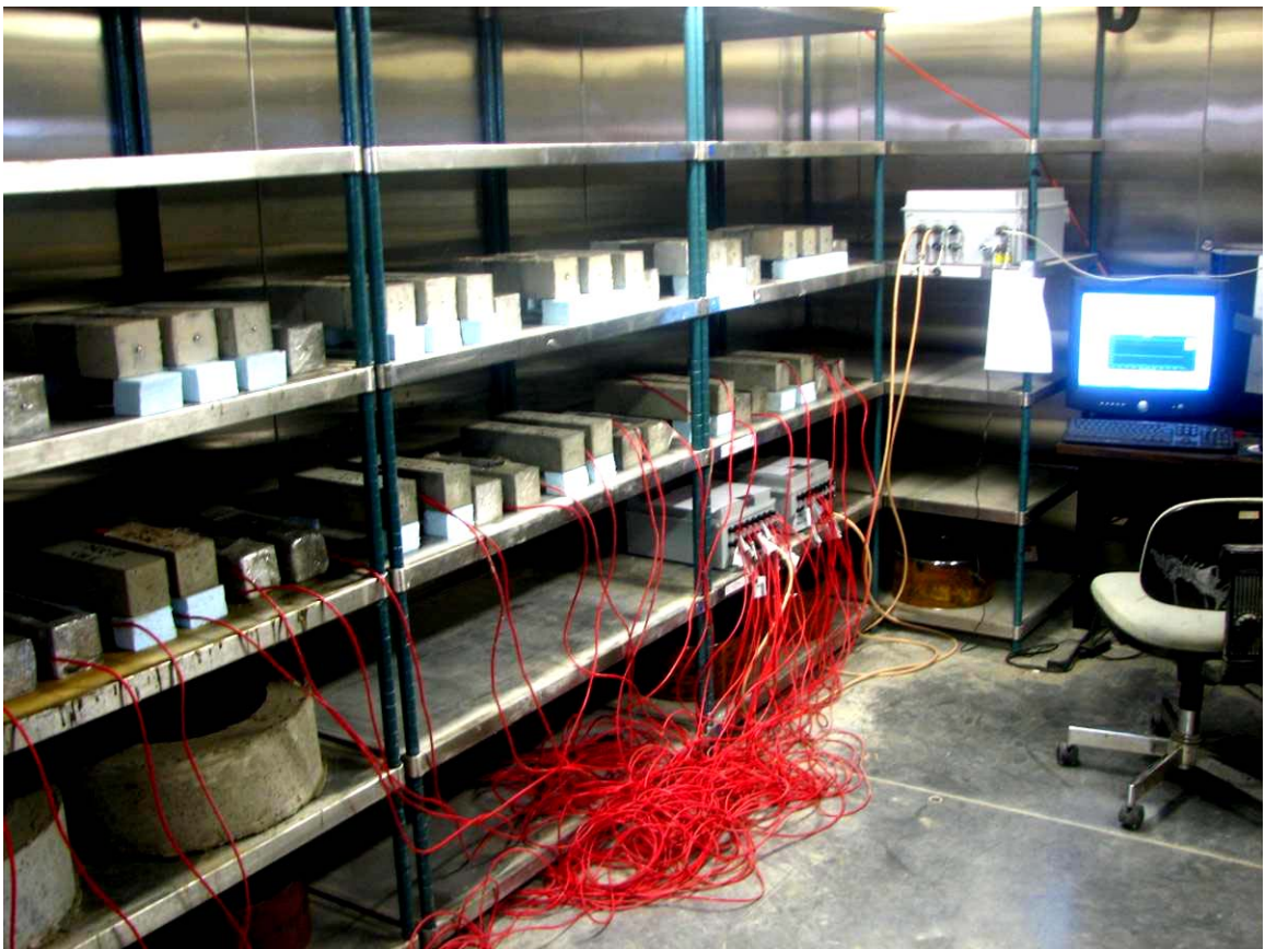
Figure6.2 Test set up for shrinkage test in the laboratory
