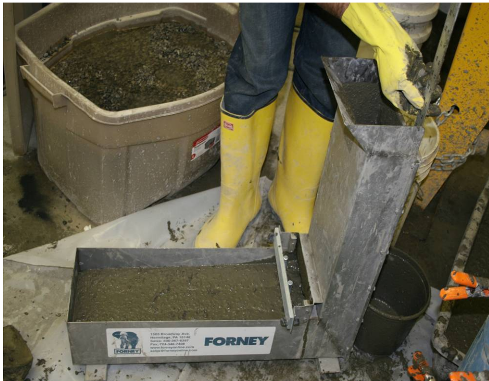
Figure 4.4 L-box test set-up (Reproduced from: The European Guidelines for Self Compacting Concrete)
