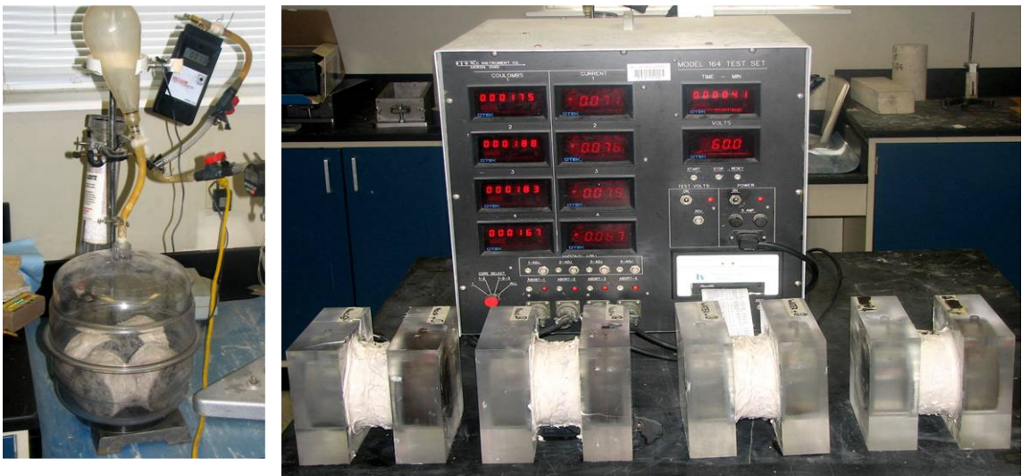
Figure 7.1 RCPT test being conducted in the laboratory
