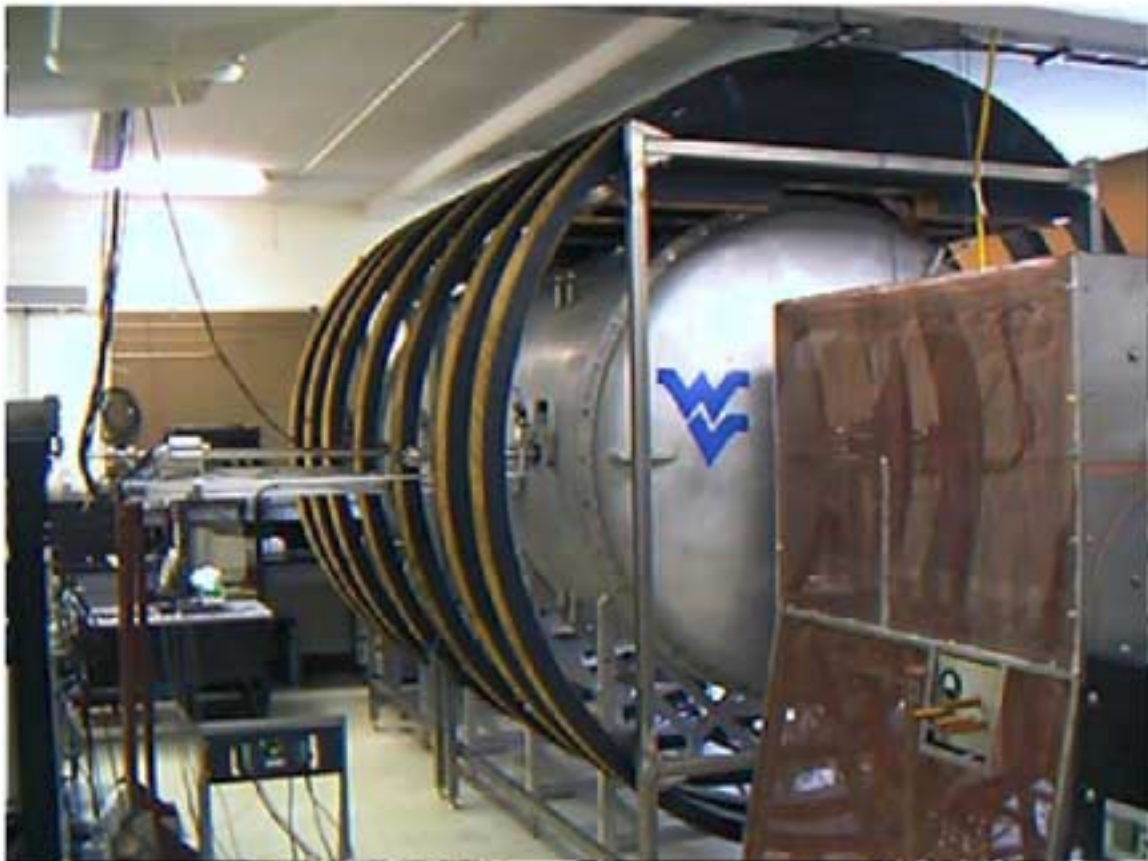
Figure 2.1 HELIX (foreground) and LEIA combined system. HELIX is enclosed in a copper Faraday cage.
