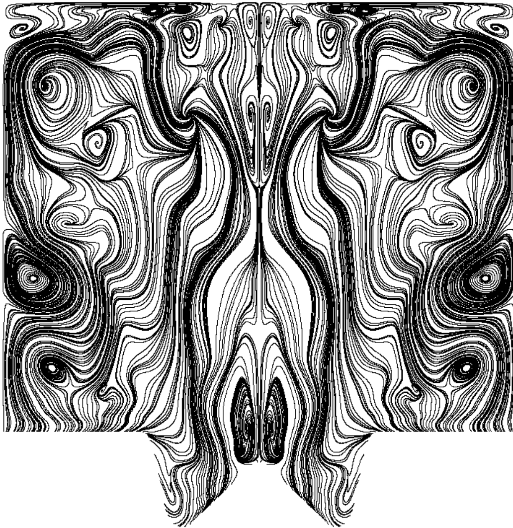
Figure 6.1 2-D Streamlines at CA 210° ATDC (with mirror image)
