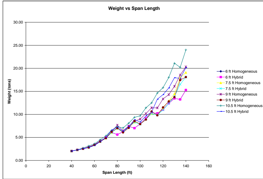
Figure 6-13 Steel Plate Girder Section Comparisons
