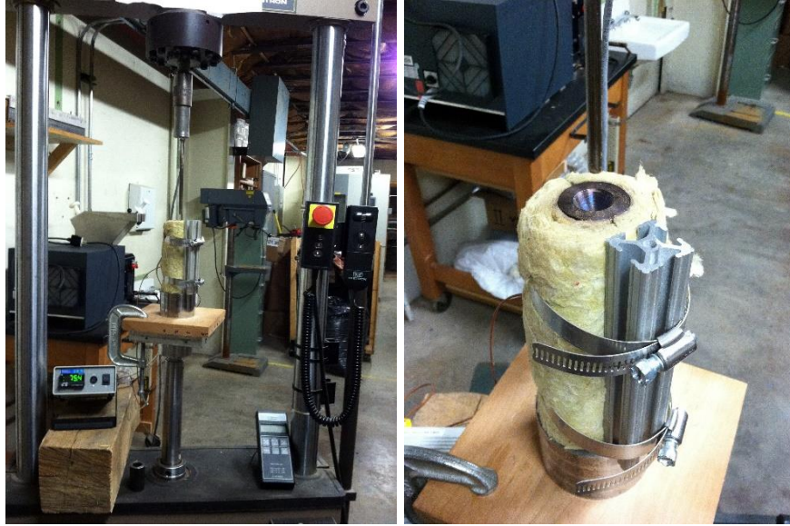
Figure 2.4 Single pellet die in place on the MTS UTM.
