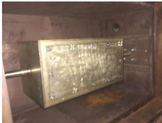
Figure 3.1 Sealed torrefaction chamber.
