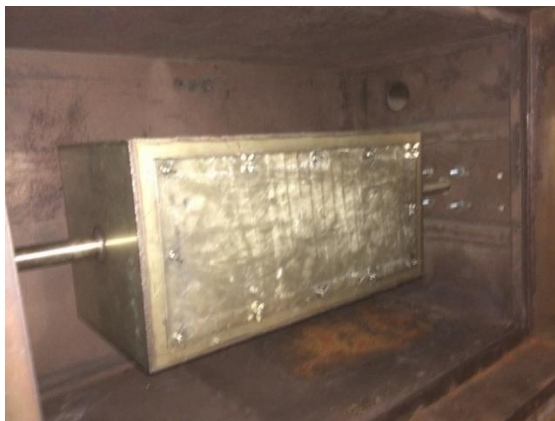
Figure 2.2 Sealed torrefaction chamber.
