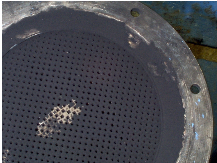
Figure 10 Upstream Face of the Rohmac/DCL DPM Control System DPM Trap Prior to Regeneration.
