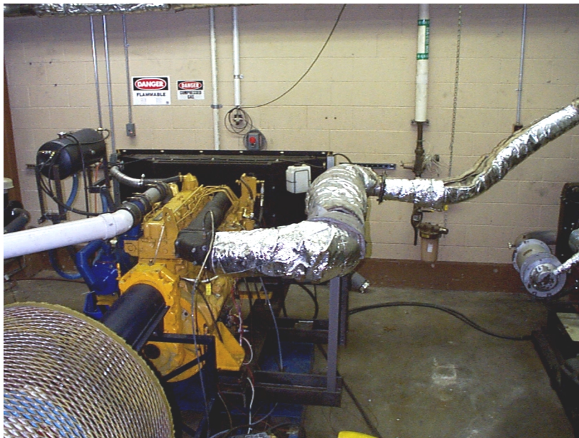
Figure 6 Caterpillar 3306 with Clean Air Systems Catalyzed DPM Trap Installed on an Eddy-Current Dynamometer Test Bed.
