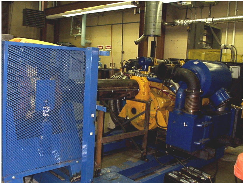
Figure 5 Caterpillar 3306 with DST Dry Scrubber System Installed on an Eddy-Current Dynamometer Test Bed.
