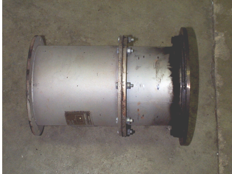
Figure 9 Side View of the Rohmac/DCL DPM Control System.
