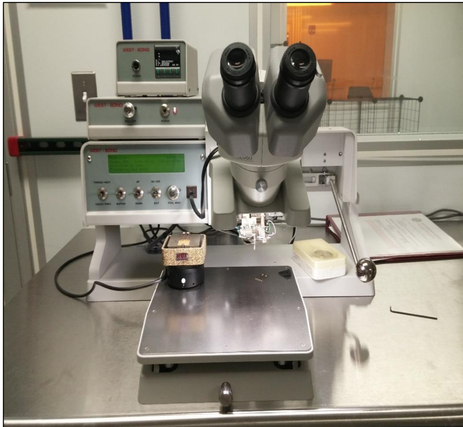
Figure 3.11: Wire bonder used for gold wire bonding between the sensor platform and the packaging.
