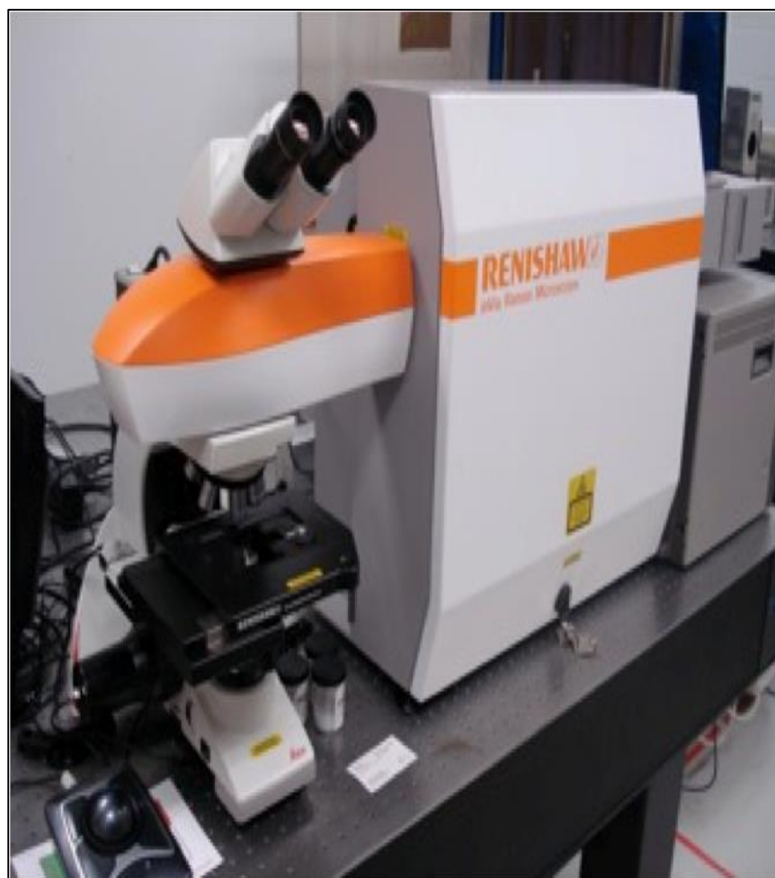
Figure 3.14: Renishaw micro-Raman spectrometer used, with the 532 nm green laser and 1 \mu\text{m} spot size.
