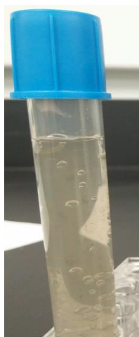
Figure 4.24: Change in color from colorless to pale yellow after 12 hours, confirming formation of silver colloid.
