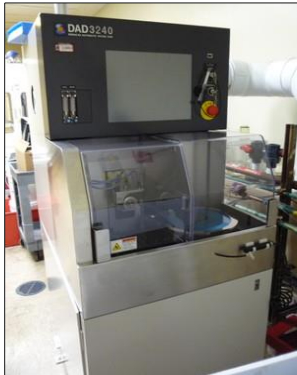
Figure 3.10: DISCO wafer dicer, capable of dicing substrates with great accuracy and minimum contamination.
