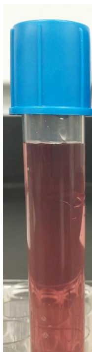
Figure 4.29: Change in color from colorless to pale purple, confirming formation of gold colloid.
