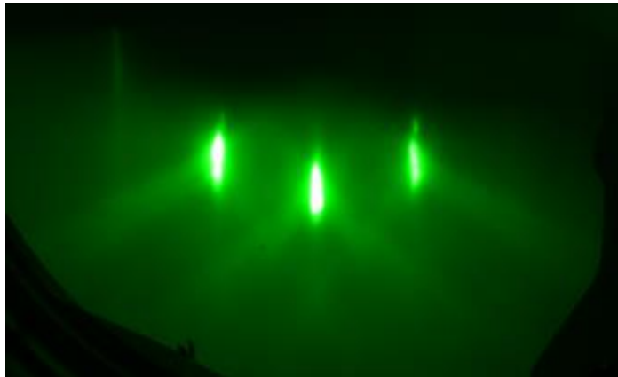
Figure 3.16: RHEED image of as received 6H-SiC (0001) surface after clean taken along [1\bar{1}0]
