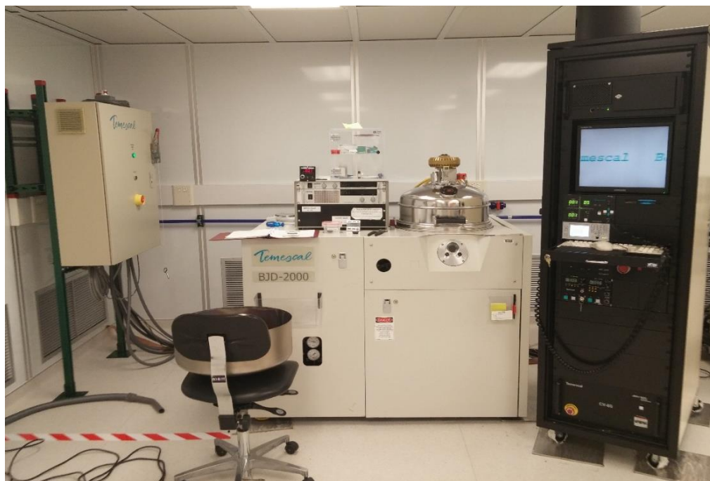
Figure 3.9: Temescal BJD200 E-beam evaporator used to deposit electrical contact in the shared Research Facilities cleanroom.
