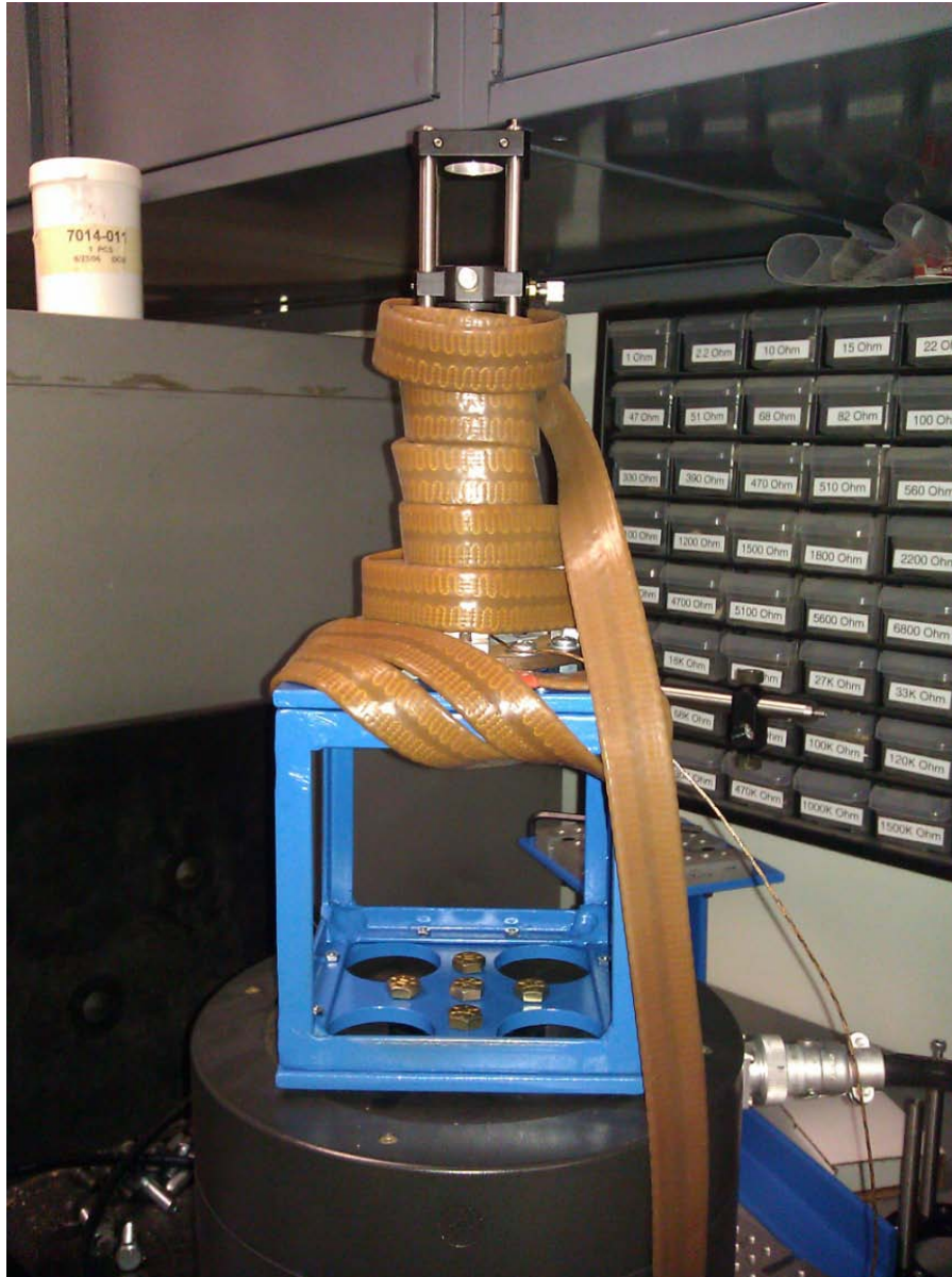
Figure 18: The laser spark plug mounted in a 90° orientation wrapped with the heat tape.
