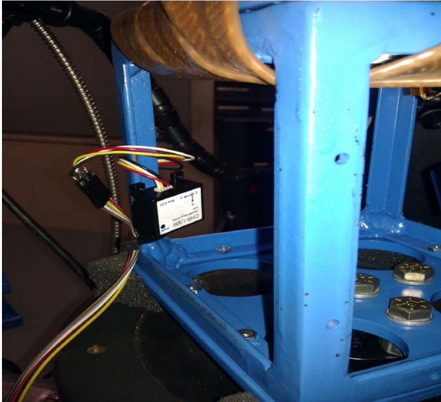
Figure 25: Accelerometer mounting location for the 0 and 90 degree mounting angles
