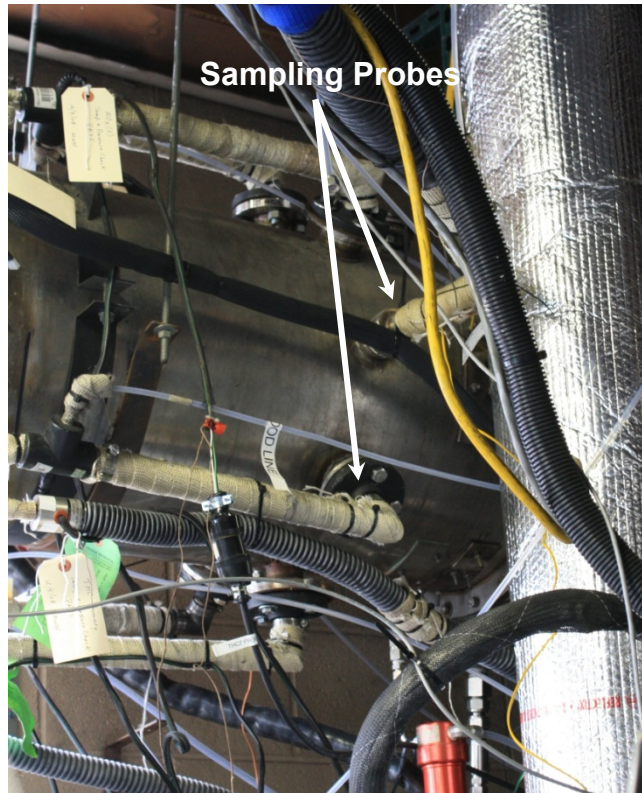
Figure 3.4 : Sampling Probes in Dilution Tunnel.
