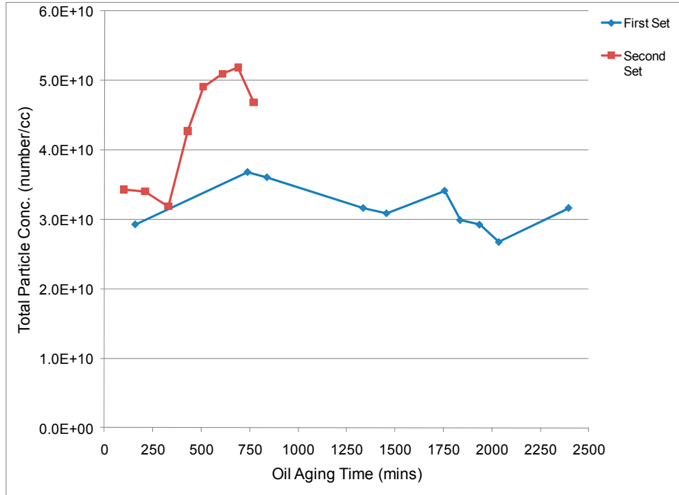
Figure 5.25 : Change in Total Particle Concentration over Aging Time.
