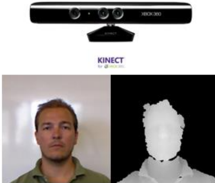
Figure 6. Kinect RGB-D image – The Kinect sensor shown above 3 is able to capture RGB and depth images at the same rate and resolution.
