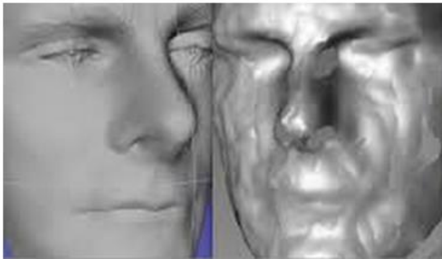
Figure 7 4 . Laser vs. RGB-D – Laser scanners can create accurate depth images (left), but the acquisition process is quite slow. RGB-D cameras can acquire depth images at 30fps, but the depth images are noisy (right).
