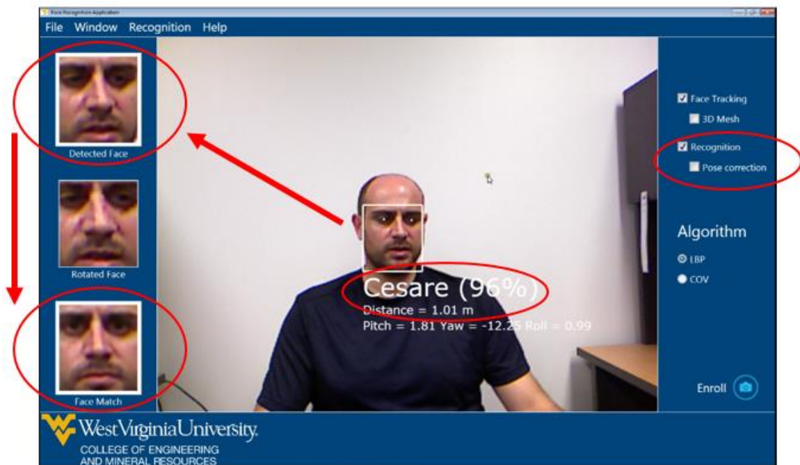
Figure 32. Face recognition software interface – The system is working without pose correction (the check box is not checked, see red ellipse on the right).
