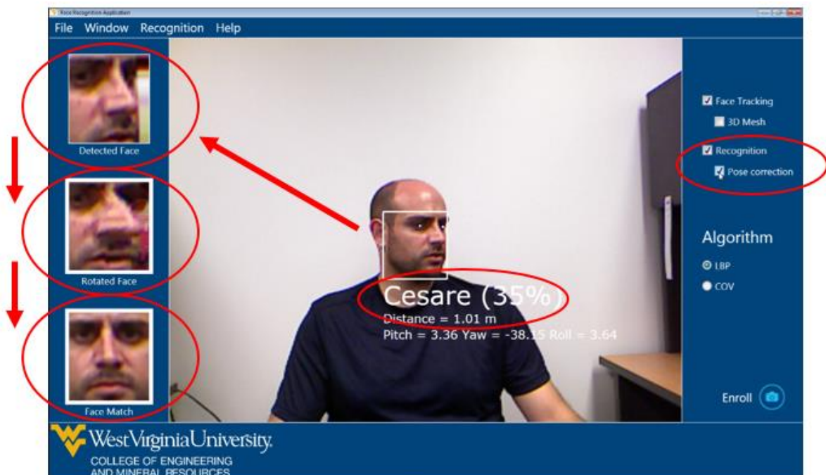
Figure 35. Face recognition success - Face recognition succeeds thanks to pose correction (see red ellipse on the right).
