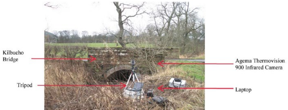
Figure 2.13: Equipment setup of Kilbucho bridge (Clark et al. 2003)
