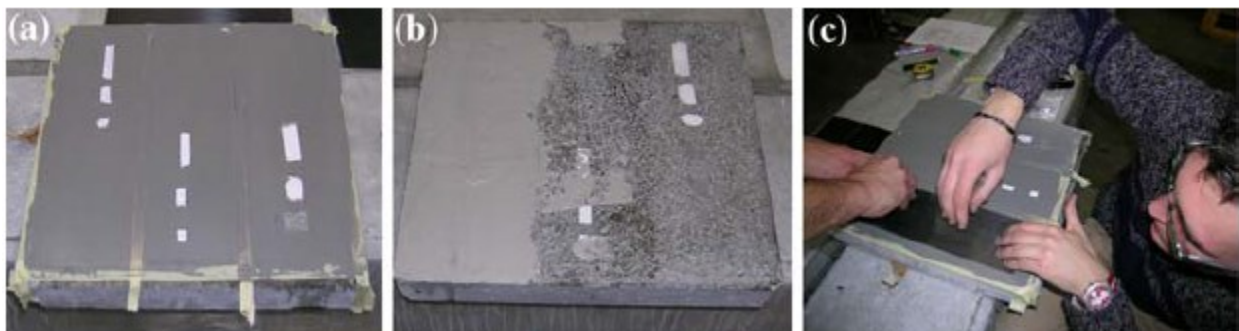
Figure 2.17: Preparation of specimens with simulated defects (a) smooth surface (b) rough surface (c) application of FRP (Valluzzi et al. 2008).
