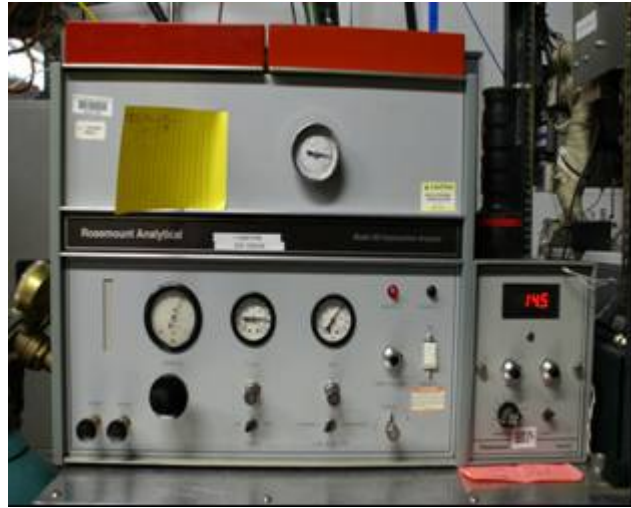
Figure 20 - Rosemount HFID Analyzer for HC
