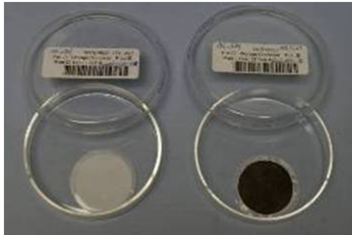
Figure 23 - PM filters (Left: Unused, Right: Engine-Out Test)
