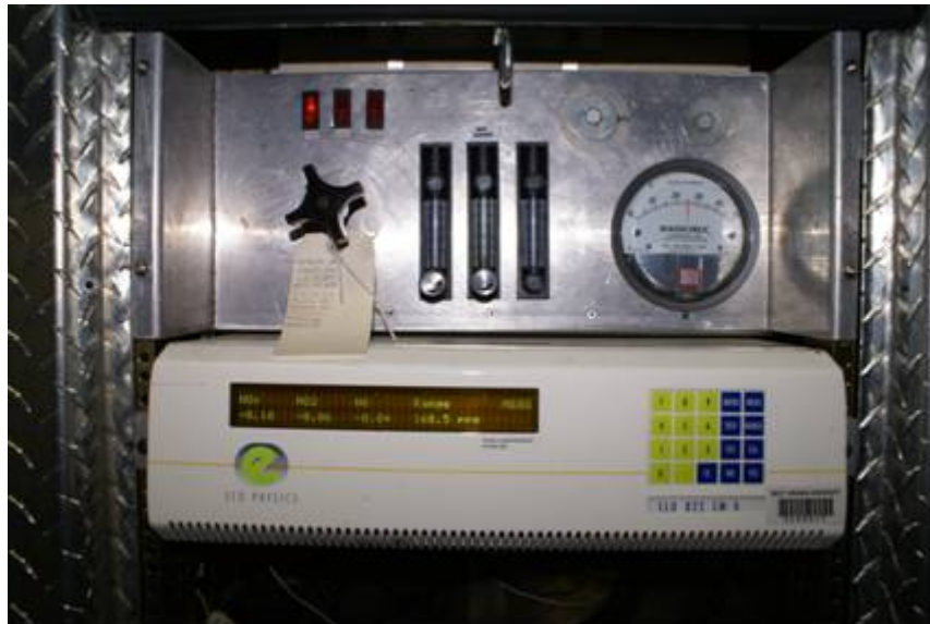
Figure 21 - Ecophysics CLD 822CMH Analyzer for NO x and NO
