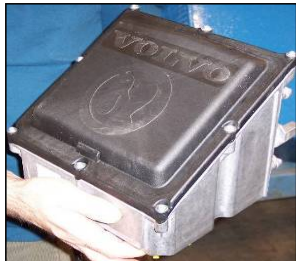
Figure 31 - Adblue Urea Pump (Front View)
