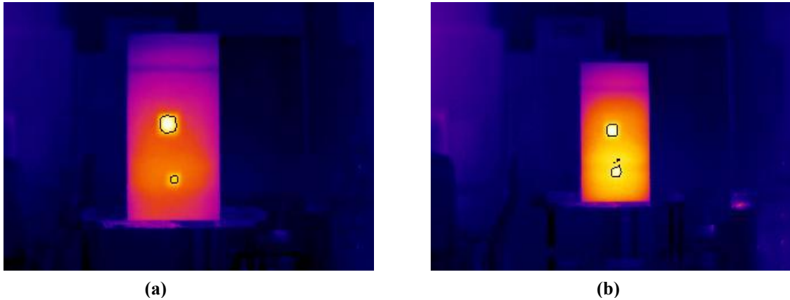
Figure 4.11: Infrared images of specimen BD1a with debonds of sizes 2"x2" and 3"x3" detected at a distance of (a) 3m (b) 4m.
