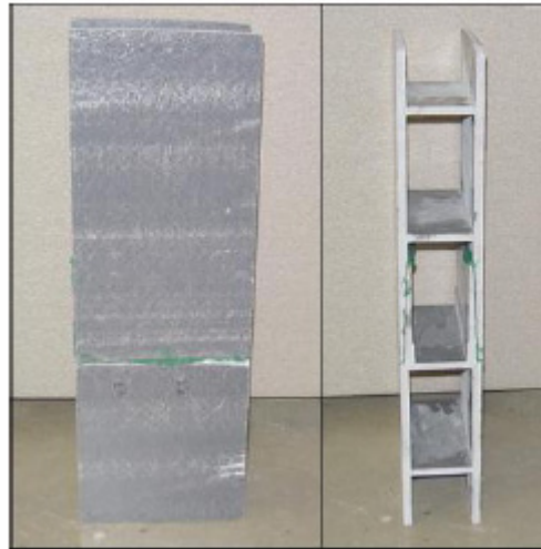
Figure 4.9: Front view and cross-sectional view of the FRP bridge deck JD1 w/o wearing surface [10].
