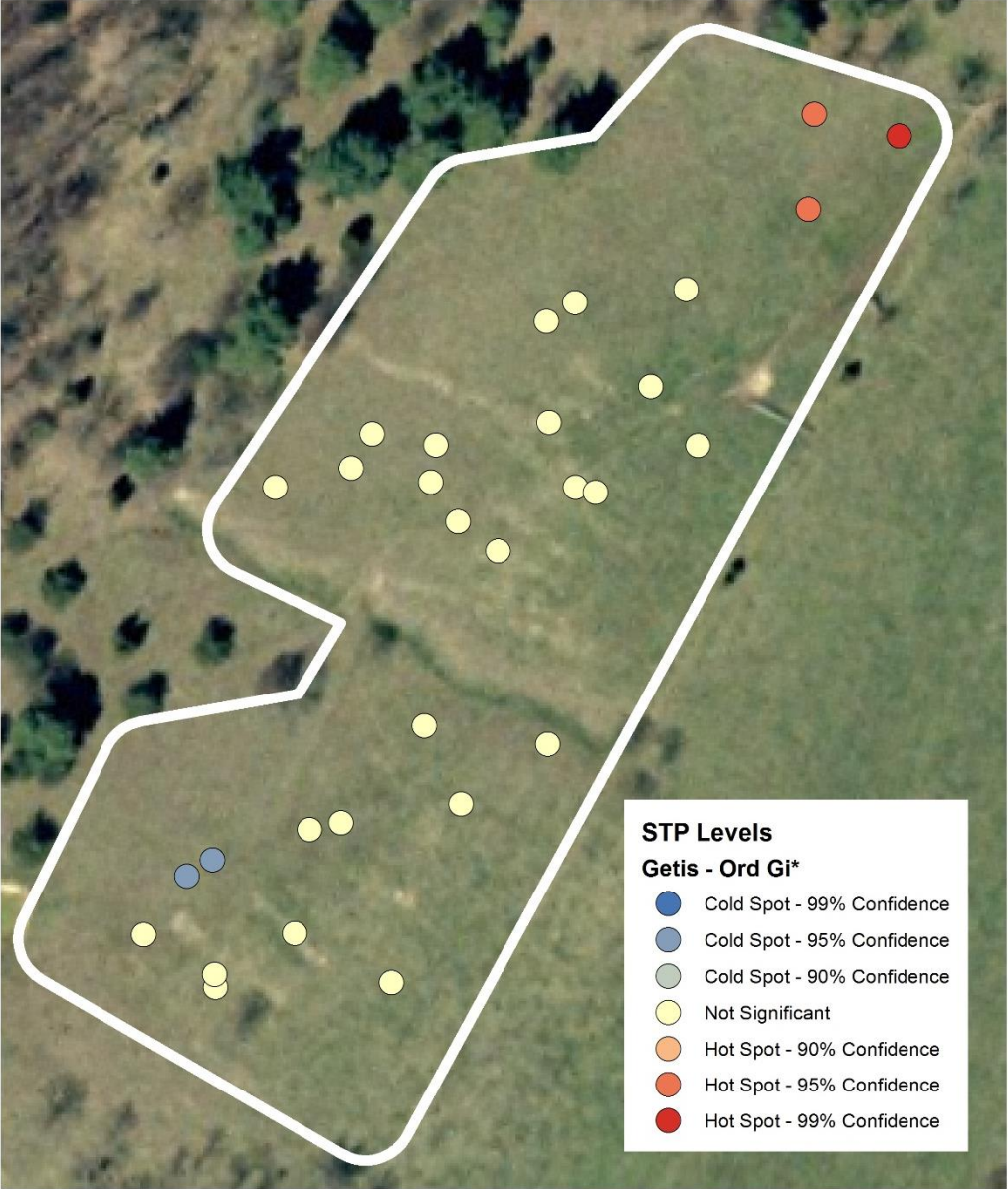
Figure 4.4 Hot spot analysis of Mehlich 1 soil test phosphorus data at location unfertilized 2 where locations with high value, surrounded by other features with high values are identified and hot spots and locations with low value, surrounded by other features with low values are identified and cold spots
