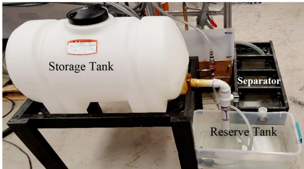
FIGURE 29 - FILTRATION AND CIRCULATION SYSTEM
