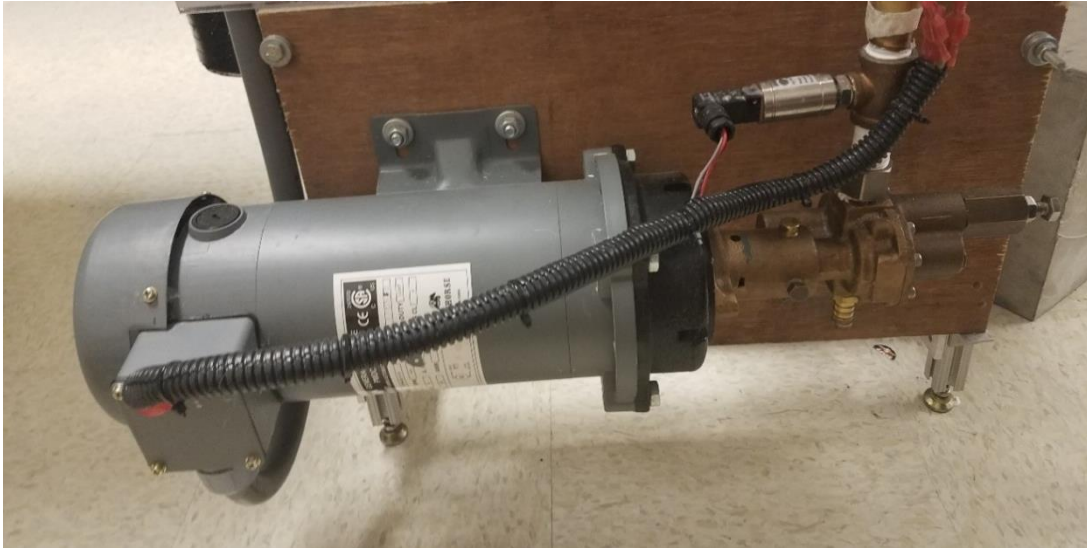
FIGURE 28 - PUMP AND PUMP MOTOR
