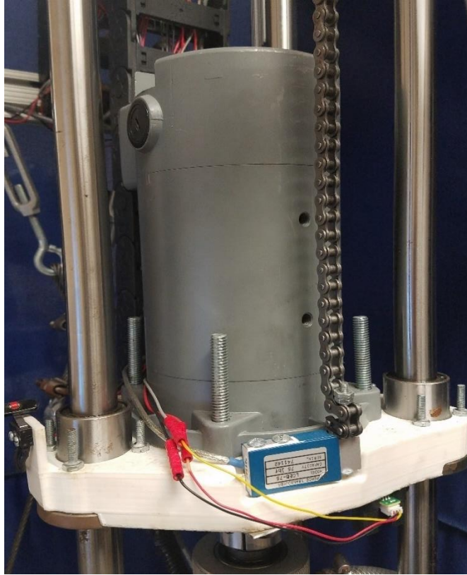
FIGURE 4 - VERTICAL GUIDE RAILS, MOTOR MOUNT, DRILL MOTOR
