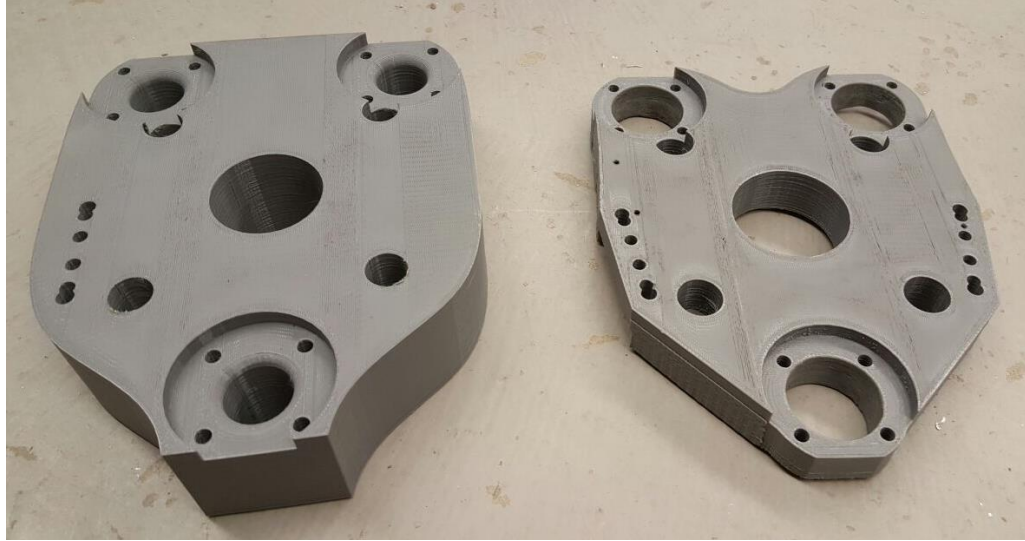
FIGURE 19 - MOTOR MOUNT ITERATIONS, EARLY (LEFT) AND LOW-PROFILE (RIGHT)
