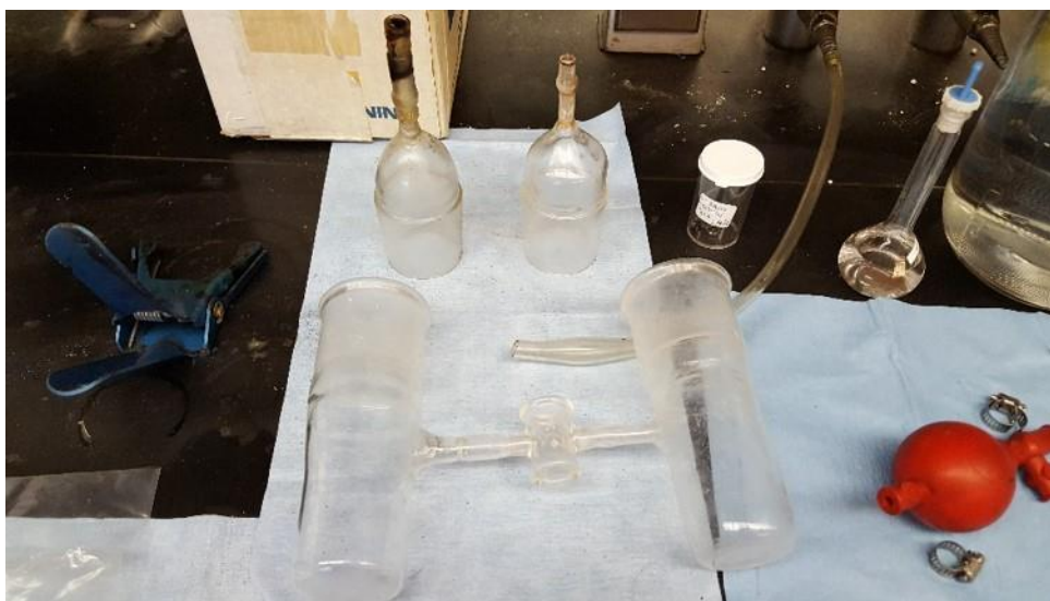
Figure 0.2 Two compartment cell with glass fritted salt bridge for solution reactions
