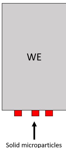
Figure 0.10 Ensembles of solid-microparticles (in red) immobilized on the surface of a solid working electrode (WE)
