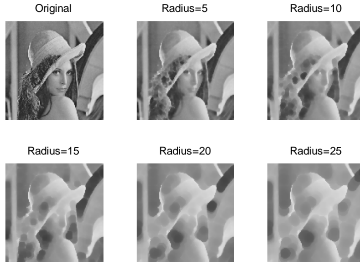
Fig. 24. Non-Flat Closing - Sphere Shaped Structure
