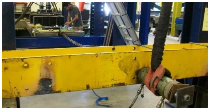
Figure 5-11. Pulling test on a top bail of the FRP gate
