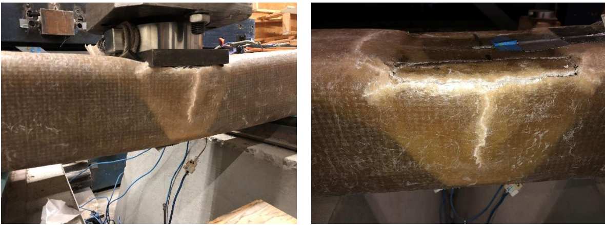
Figure 7-64. Failure in HFB beam, (a) web buckling/splitting, (b) punching shear failure
