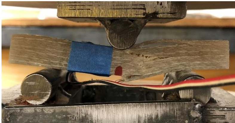
Figure 6-22. Failed transverse GFRP laminate under three-point bending
