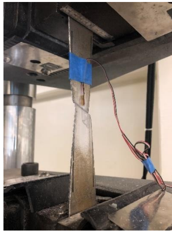
Figure 6-4. Tensile failure on, (a) Steel plate, (b) GFRP laminate
