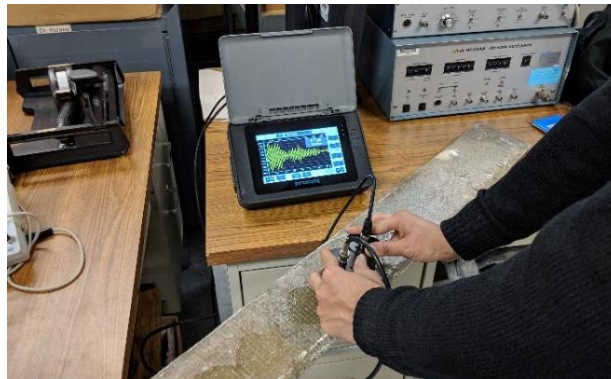
Figure B-7. Ultrasound testing on hybrid GFRP-steel laminate via indirect transmission
