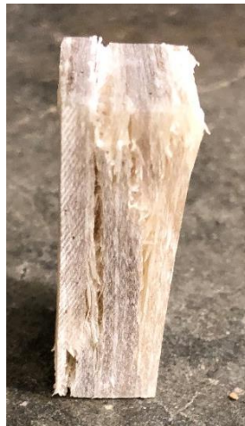
Figure 6-12. Failure of GFRP specimen under compressive stress
