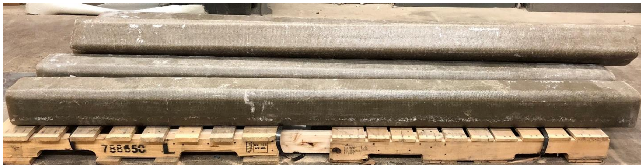
Figure 4-4. Control GFRP and GFRP-steel hybrid box beams
