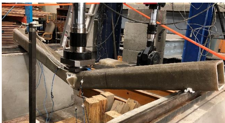
Figure 7-21. Failure of a hybrid HAB beam under fatigue at a load range of 10-15 kip at 2.5 Hz
