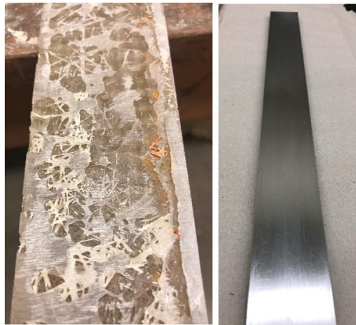
Figure C-1. Separated GFRP-steel bonded surfaces
