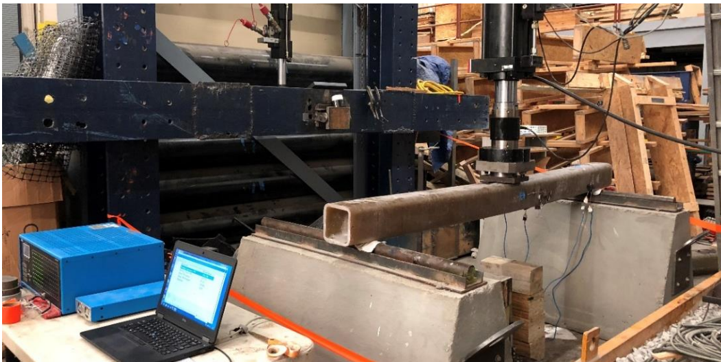
Figure 7-9. Fatigue testing under 3-point loading at a span of 84 in.
