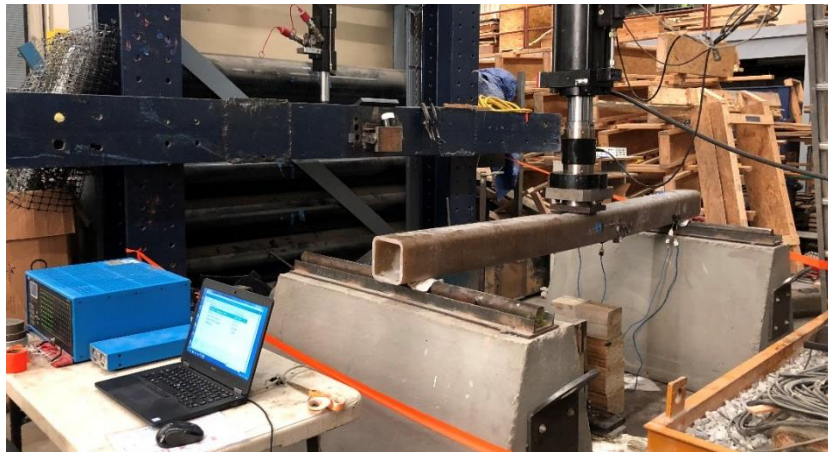
Figure 4-9. Three-point bending setup for testing a box-beam
