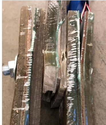
Figure 10-13. Failure in GFRP-steel hybrid member with single-row bolted connection
