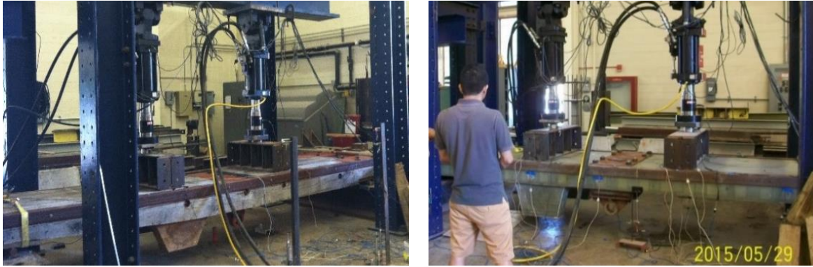
(a) (b) Figure 5-9. Bending tests: (a) on timber wicket gate, (b) on GFRP-steel wicket gate
