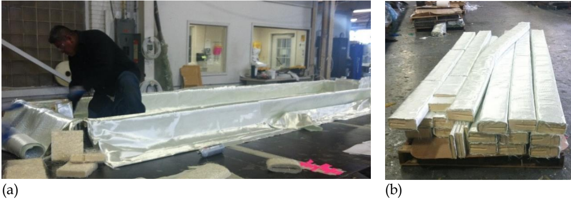
Figure 4-2. (a) Manufacturing of hybrid GFRP panel, (b) GFRP web cores
