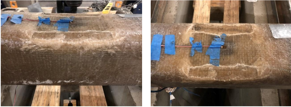
(a) (b) Figure 7-60. HWB beam failure: (a) flange-web junction crack, (b) transverse shear failure
