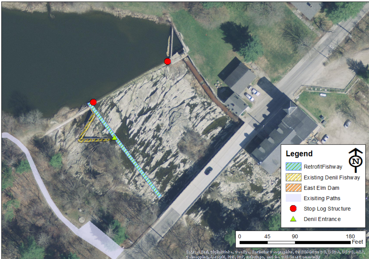
Figure 11: Possible Bridge Street dam site alignment and dimensions of new Denil fishway to meet USFWS criteria (Table 4).
