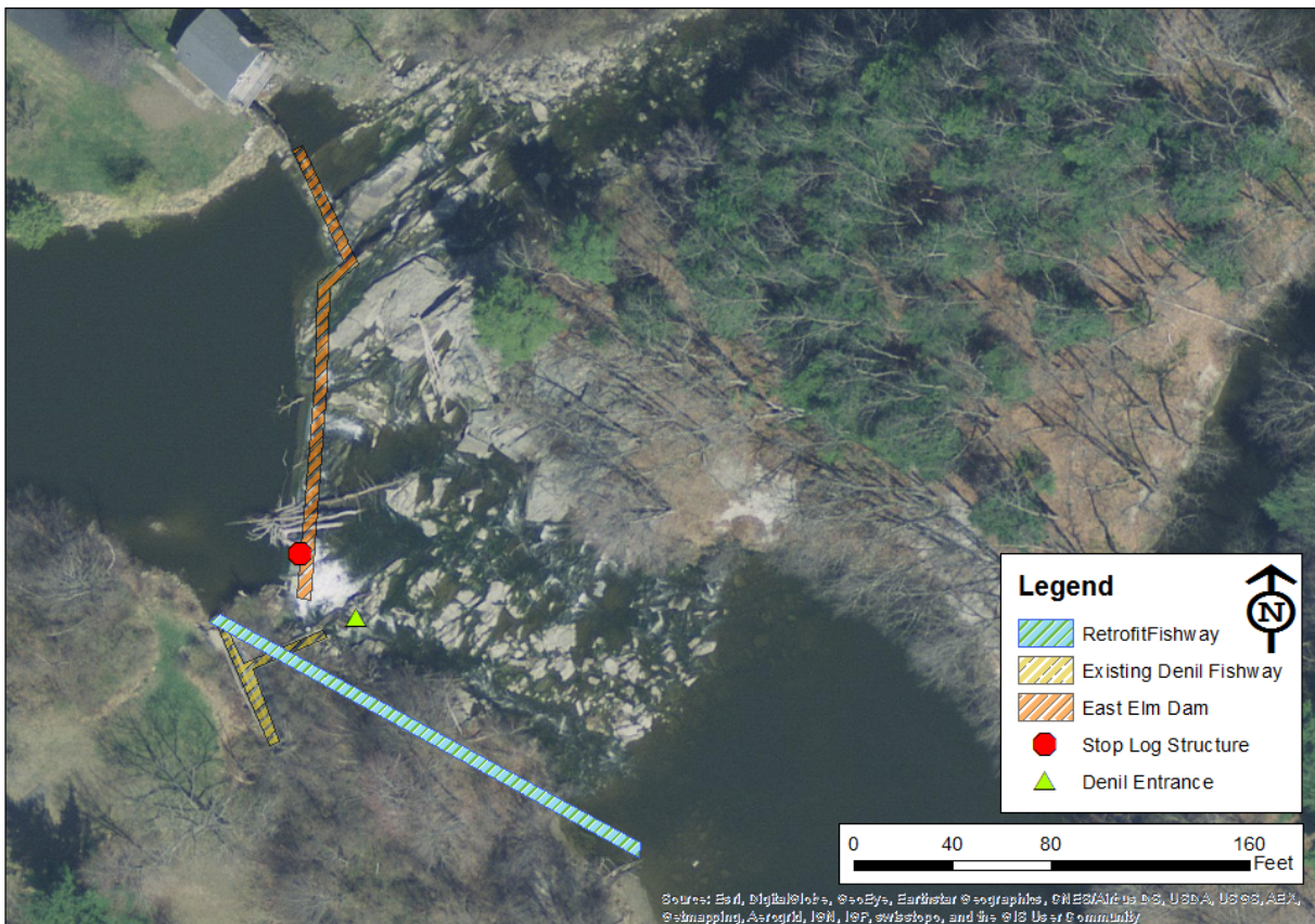
Figure 14: Location and dimensions of proposed retrofit of existing East Elm Street Denil fishway to meet USFWS criteria (Table 4).
