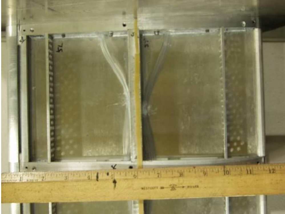
Figure 4.4: Internal Structure of the Blade Segment [Angle, 2008]
