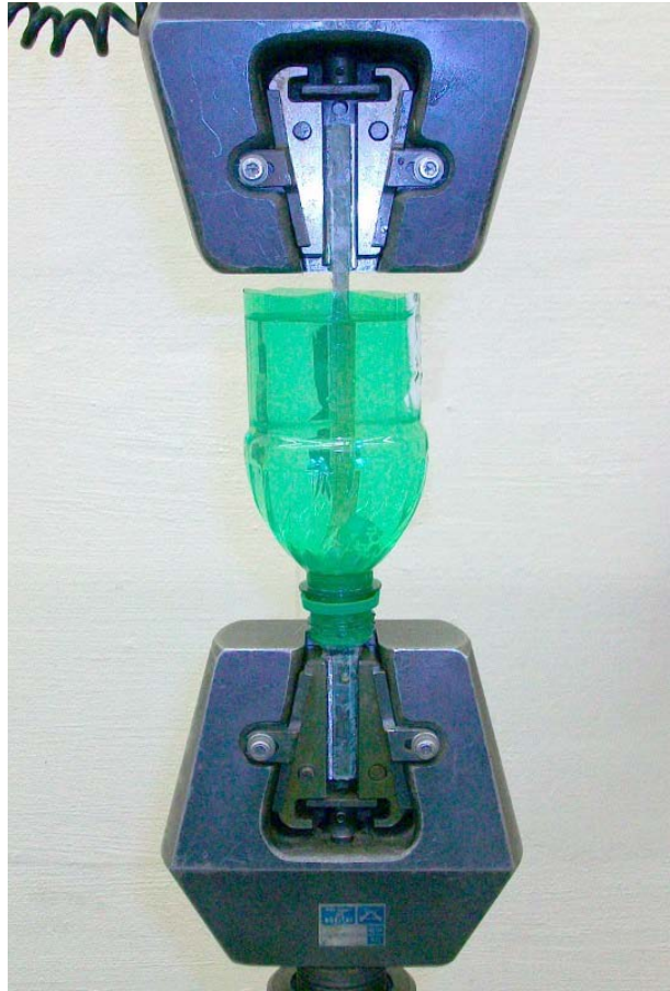
Figure 3-14 - Tension Clamps (Shown with Water Containment Bottle)
