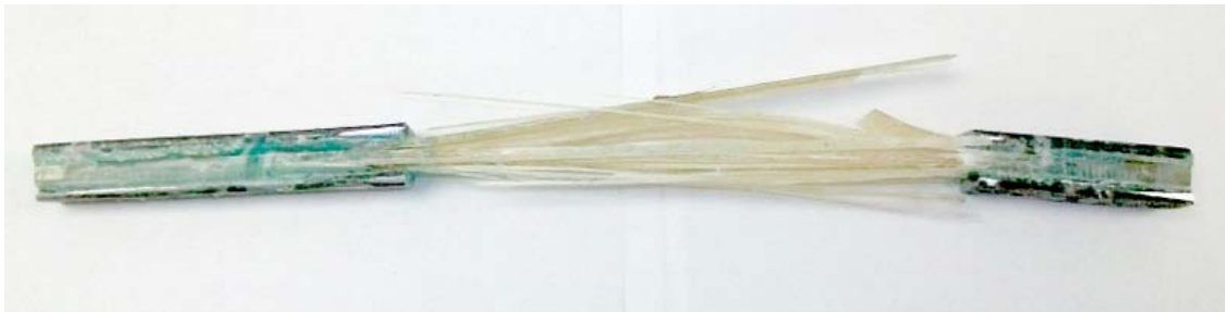
Figure 3-27 - Failed Static Tensile Sample (2.1)
