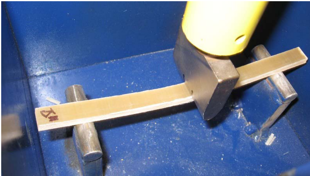
Figure 3-15 - Bending Test Fixture with Sample
