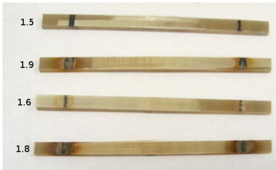
Figure 3-29 - Failed Bending Fatigue Samples (Tension Side)
