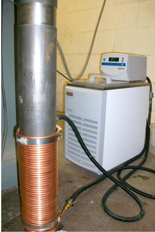
Figure 3-21 - Elevated Temperature / Pressurized Immersion Chamber
