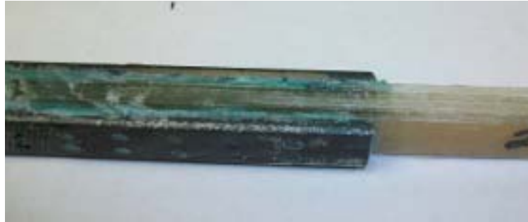
Figure 3-3 - Steel tabs attached to sample
