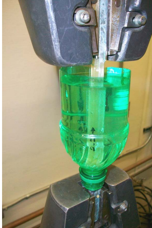
Figure 3-4 - Completed water containment sample on testing machine
