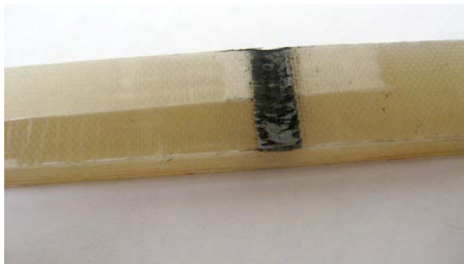
Figure 3-28 - Depressions at Supports on Bending Fatigue Samples
