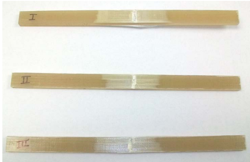
Figure 3-24 - Failed Static Bending Samples
