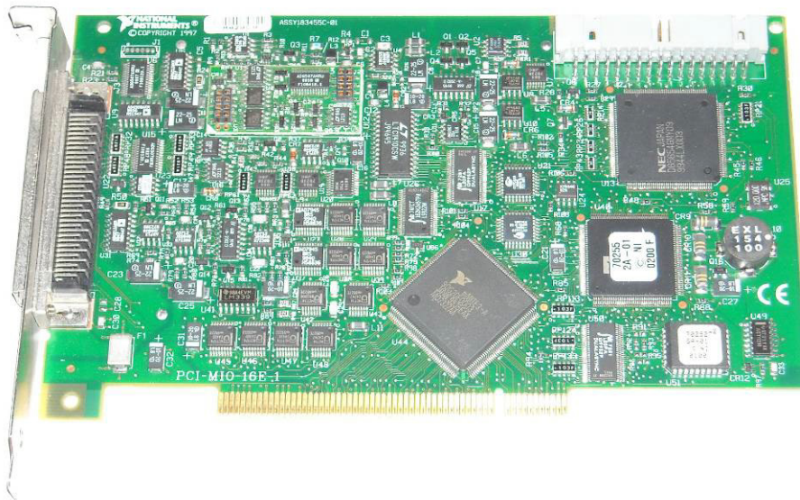
Figure 93: NI PCI-MIO-16E-1, one of two DAQ cards utilized.
