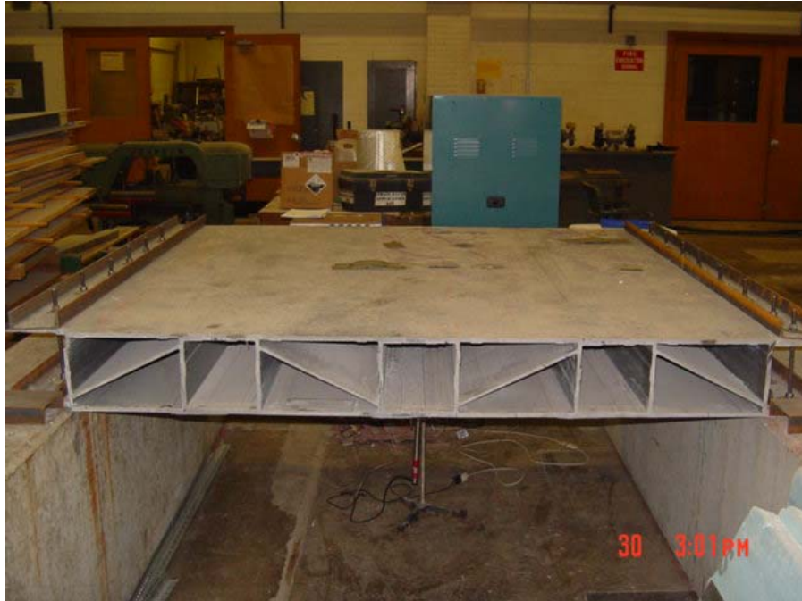
Figure 4.4: Test Set-Up for SSFF Boundary Condition.
