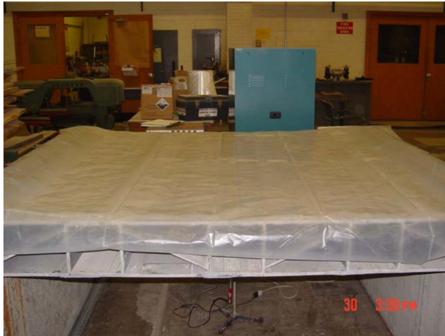
Figure 4.14: Plastic Sheet Covered the Entire Top Surface.
