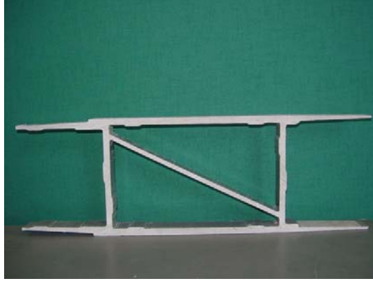
b) 8 inch Deep FRP Deck
