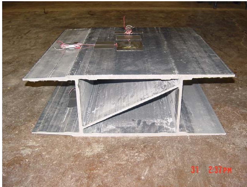
Figure 3.2(a): Specimen #2 (A Module of 8 in. FRP Deck with 24 inches in Length).
