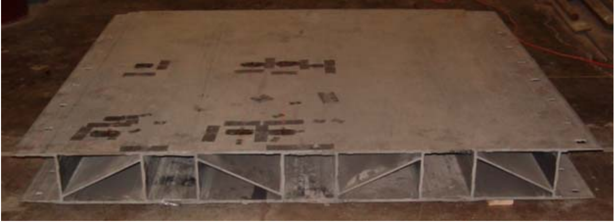
Figure 4.3: A 8 inch Deep FRP Deck Specimen.
