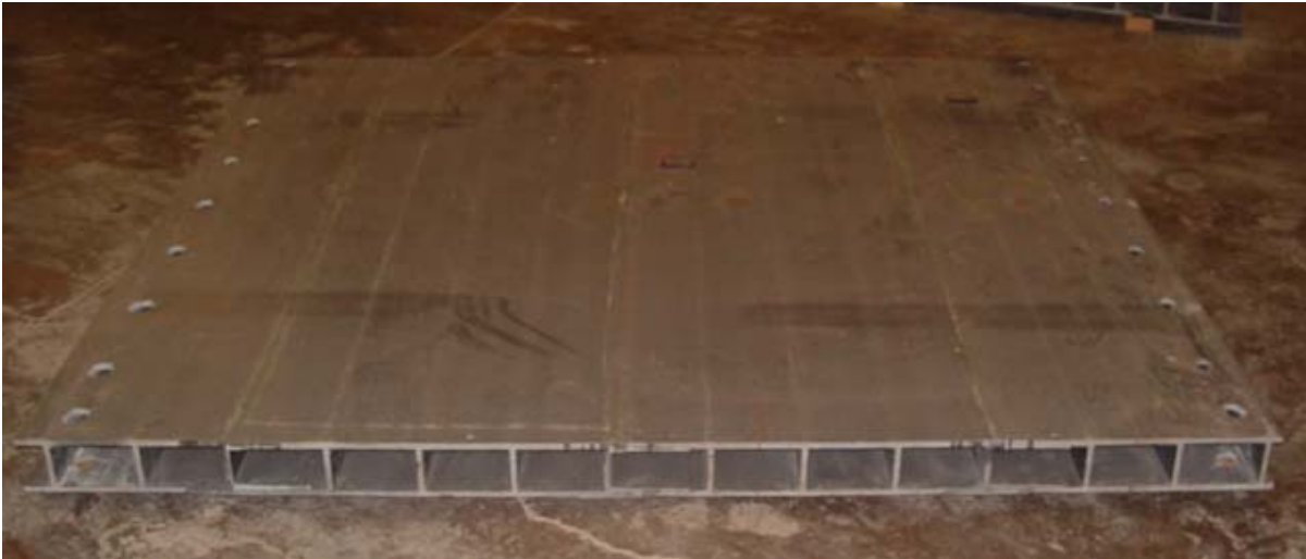
Figure 4.2: A 4 inch Deep FRP Deck Specimen.
