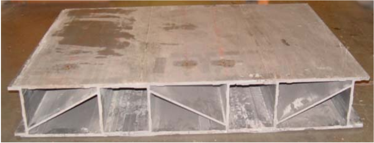
Figure 3.4(a): Specimen # 4 (Three Modules of 8 in. FRP Deck with 3 ft. in Length).
