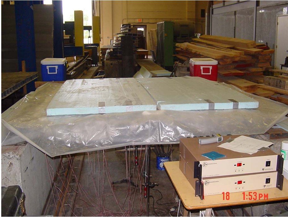
Figure 4.17: Insulation Sheets Covered on the Top of Dry Ice.
