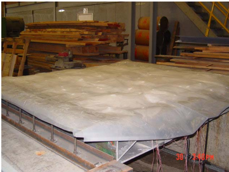
Figure 4.16: Covering the Dry Ice with Plastic Sheet.
