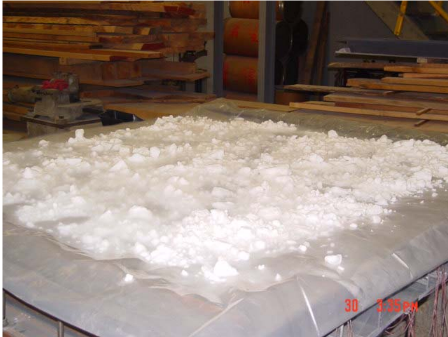
Figure 4.15: Applying Dry Ice on the Top Surface of FRP Deck.
