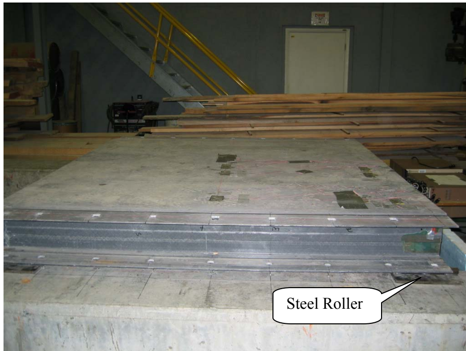
Figure 4.6: Test Set-Up for FFFF Boundary.
