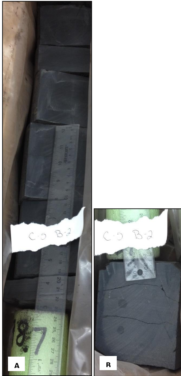
Figure A-26. Picture of Core 5, Box & Bag 2. A. The upper portion of core to the missing section. B. The lower portion of the core after the missing section
