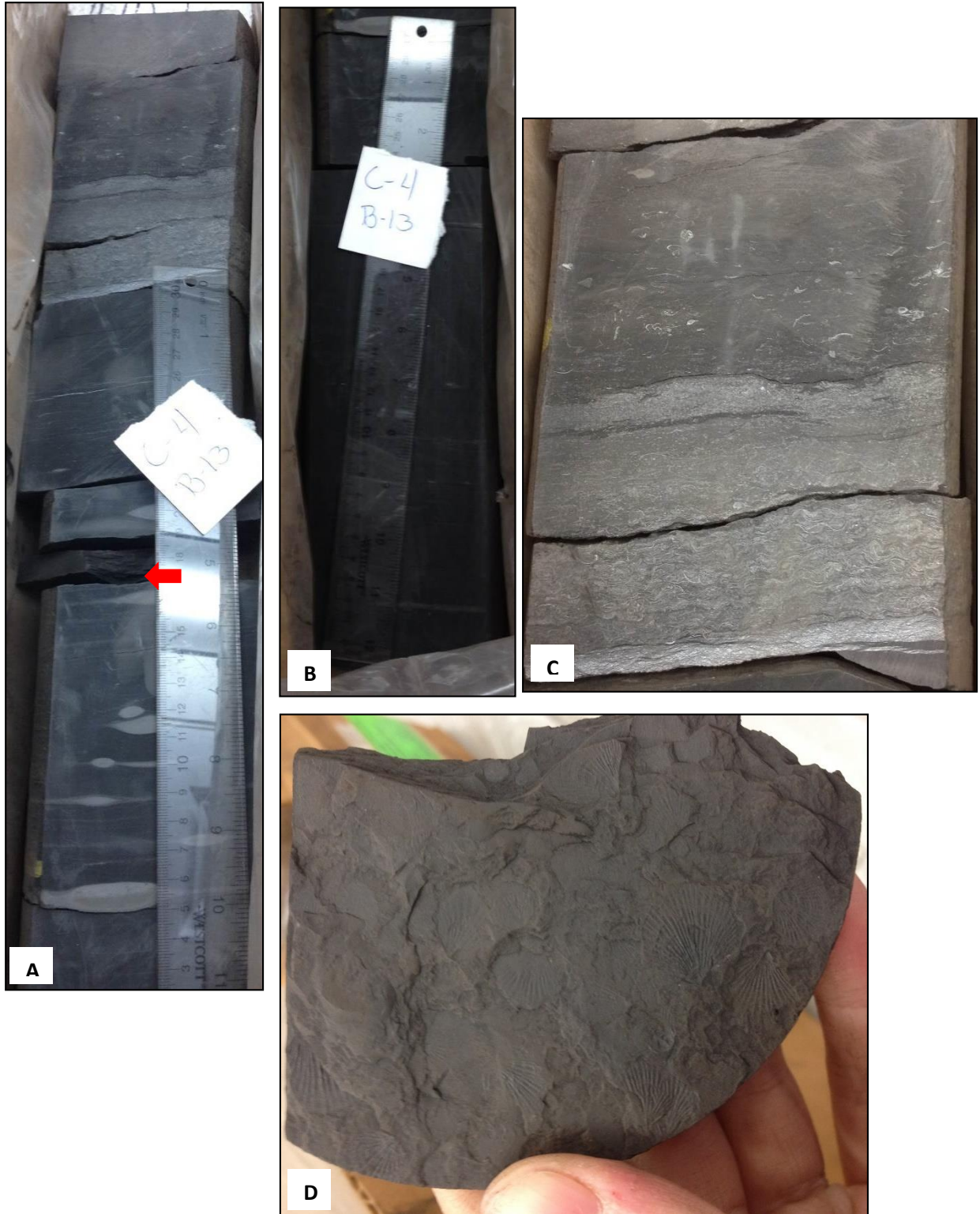
Figure A-17. Picture of Core 4, Box & Bag 13 and features within that section. A. The upper portion of the core. B. The lower section of the core (continuing from where picture A stopped). C. A zoomed in image of the turbidity current. D. Image of seashells along bedding planes (location indicated by red arrow in image A).
