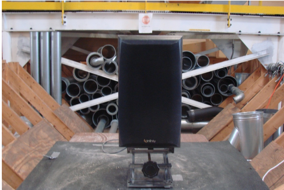
Figure 4. Speaker Location on Metal Pedestal
