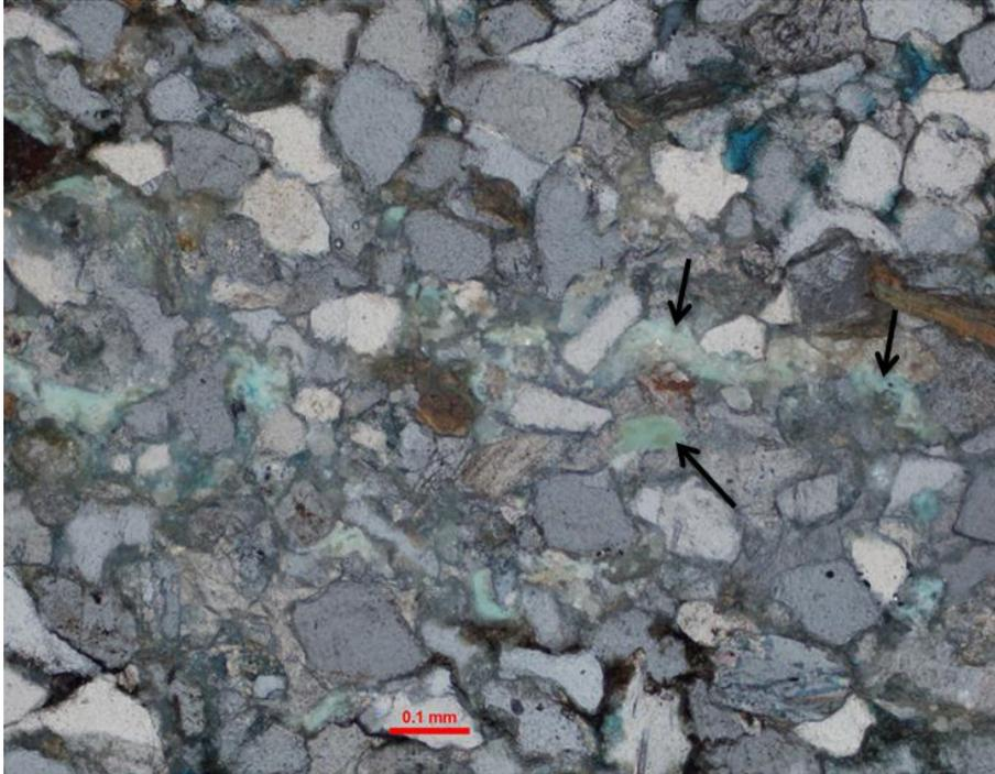
**Figure 19. Photomicrograph of thin section 3232-10815 showing the blue titanium oxide mineral under reflected light.**
