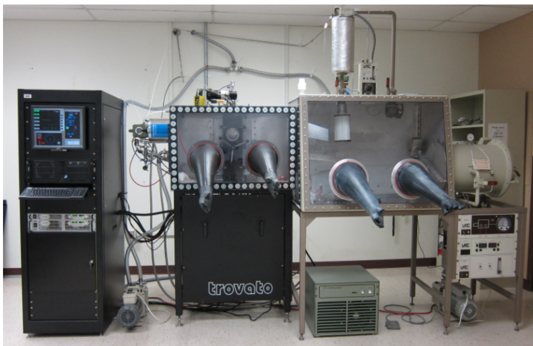
Figure 6.1 – The academic series research evaporator from Trovato Mfg., Inc with the attached glove box.
