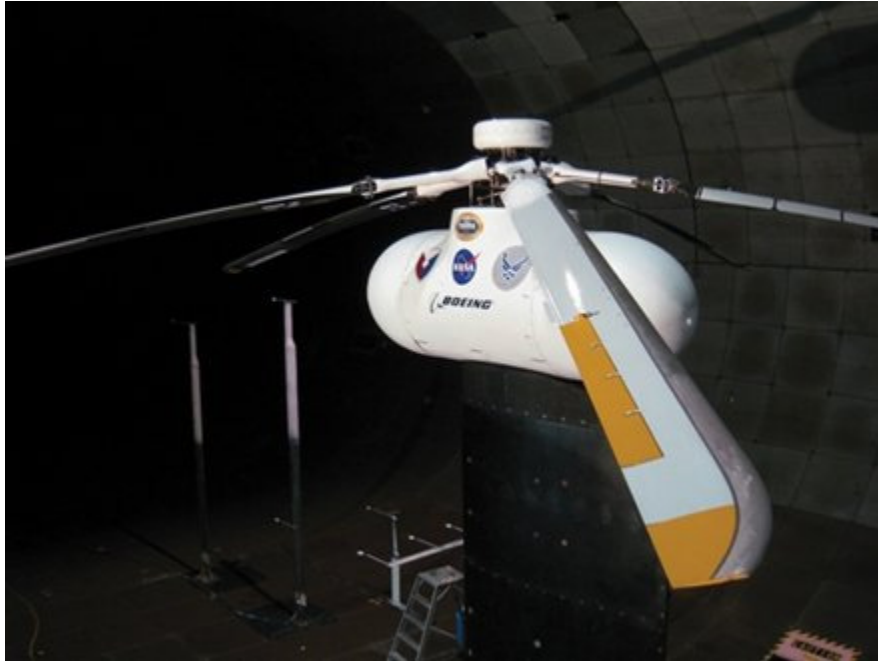
Figure 15 Active plain trail edge flaps on the SMART rotor 54
