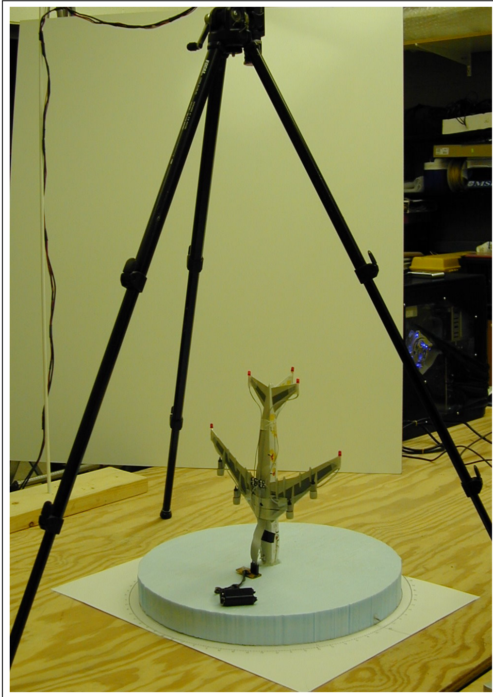
Figure 4.6: Tripod and Camera In Position Over The Model Tanker
