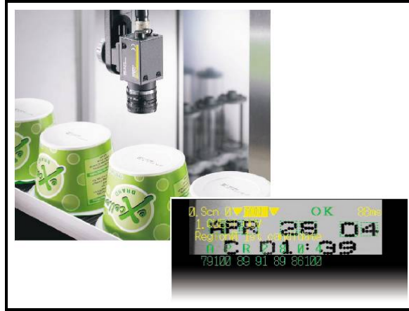
Figure 2.2: MV Inspection System for Date and Time on Yogurt Cups 49
