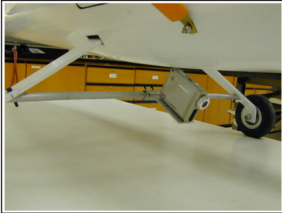
Figure 4.17: Close Up View of the DV4000 Camera Mounted on the Cessna 152
