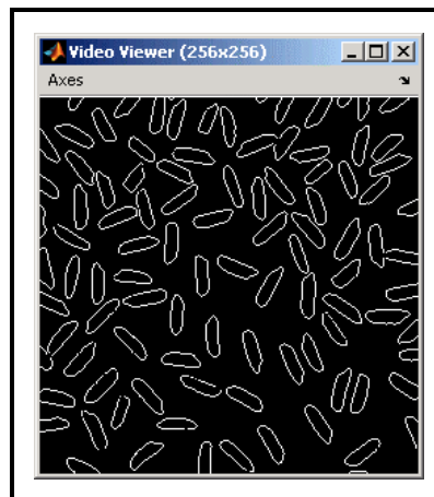
Figure 3.13: Visual Example of Sobel Edge Detection Final Product 60
