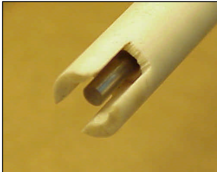
Figure 3b: Picture of the baffled Langmuir probe.
