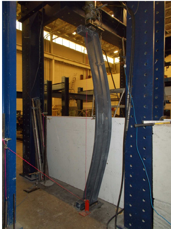
Figure 3-10: Sample Failure Modes: Local Instability in FRP 4x1.25-4 Bush-Col 1 (Top Left), Lateral-Torsional Buckling in FRP 4x1.375-6 Bush-Col 3 (Top Right), Local Instability/Material Rupture in FRP 5.5x1.5-8 Bush-Col 2 (Bottom)
