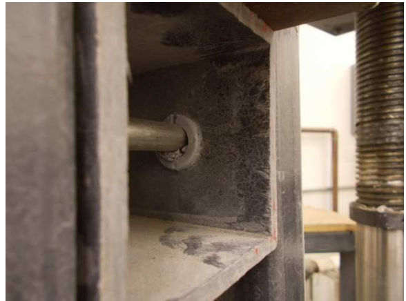
Figure 3-16: Bearing Failure of FRP 3.5x1.5 with Bushing in Column Only
