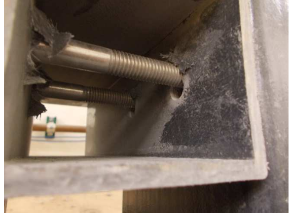
Figure 3-15: Bearing Failure of FRP 6x1.625 with No Bushing
