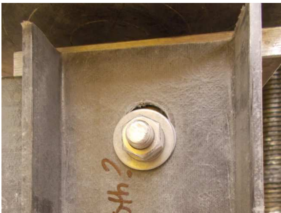
Figure 3-17: Bearing Failure of FRP 4x1.375 with Bushing in Both Column and Tie
