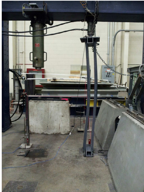
Figure 3-8: Sample Failure Modes: Local Instability/Lateral-Torsional Buckling in FRP 3.5x1.5-4 No #1 (Top Left), Local Instability/Material Rupture in FRP 4x1.375-4 No #2 (Top Right), Local Instability in FRP 6x1.625-6 No #1 (Bottom)
