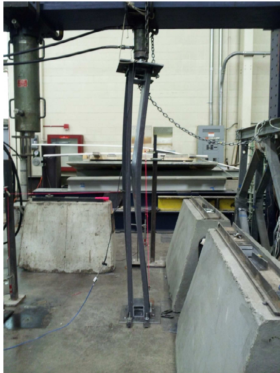
Figure 3-12: Sample Failure Modes: Material Rupture in FRP 3.5x1.5-4 Bush-Both 2 (Top Left), Local Instability in FRP 4x1.375-6 Bush-Both 2 (Top Right), Local Instability/Lateral-Torsional Buckling in FRP 5.5x1.5-6 Bush-Both 1 (Bottom)
