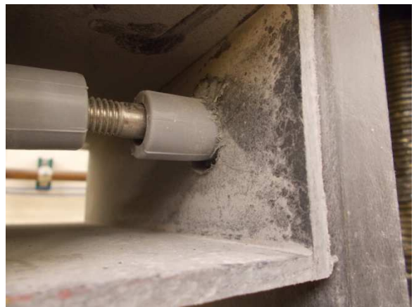
Figure 3-17: Bearing Failure of FRP 4x1.375 with Bushing in Both Column and Tie
