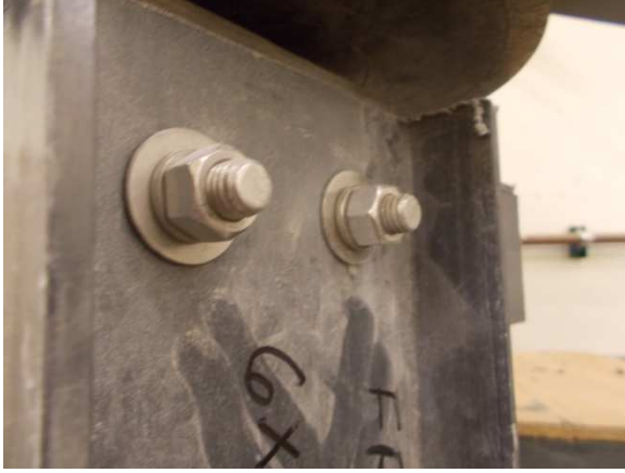
Figure 3-15: Bearing Failure of FRP 6x1.625 with No Bushing
