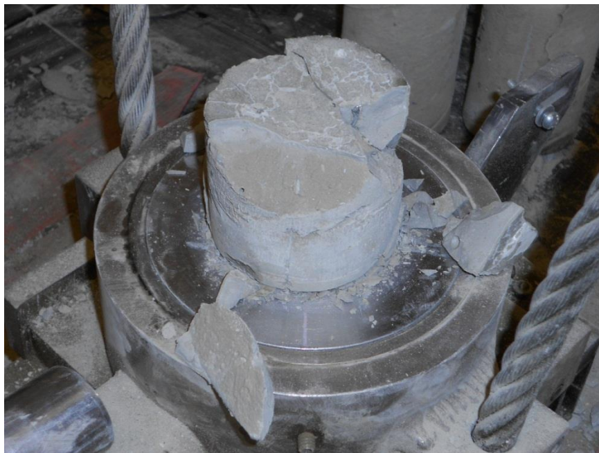
Figure 5.4: Sample B01 Post-Test. Fractures propagating along embedments.
