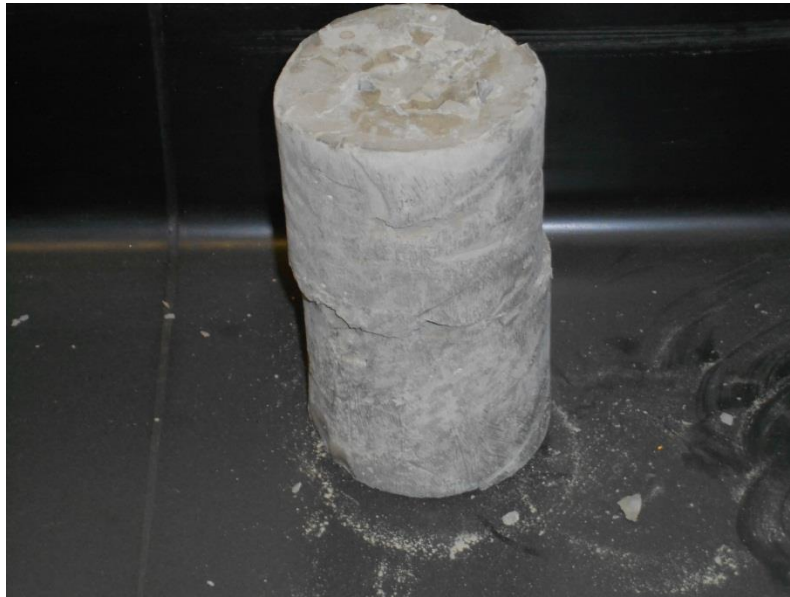
Figure 5.5: Sample C03 Post-Test. Embedments solid with fracture confined to plane of shear force.
