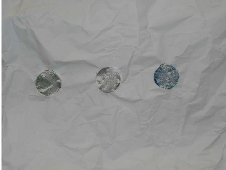
Figure 5.21: Pigmented grout samples in simulated coal face with rock dust or light-colored rock.
