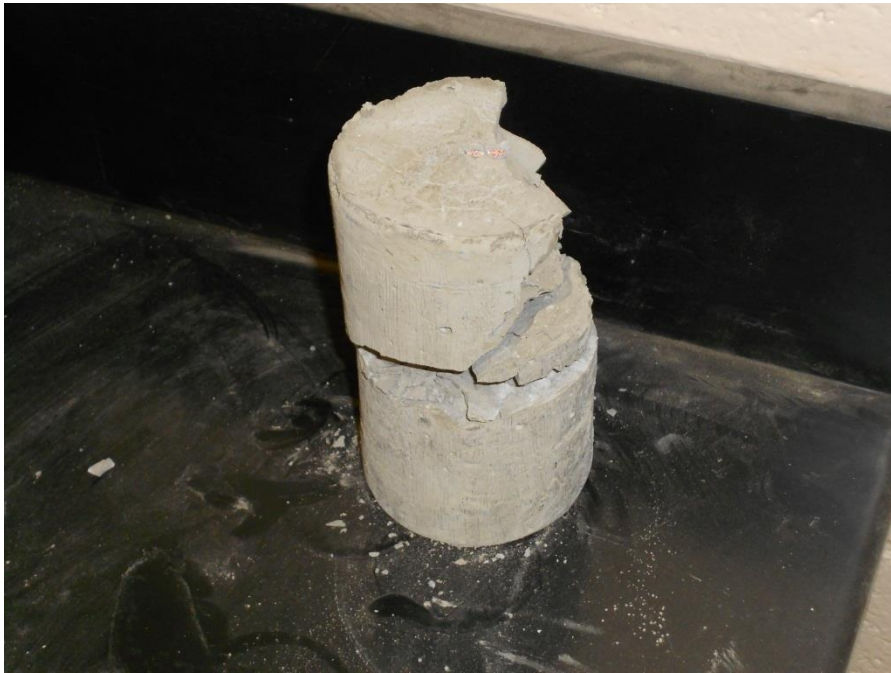
Figure 5.11: Sample F04 Post-Test. Angular cracks from plane of direct shear load.
