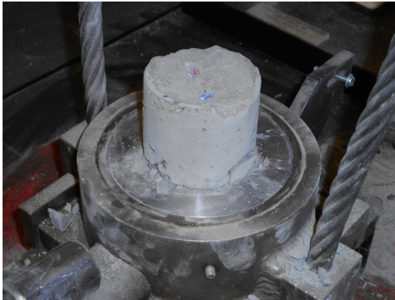
Figure 5.8: Sample E05 Post-Test. Before removal from platen. Shows structure of fracture.
