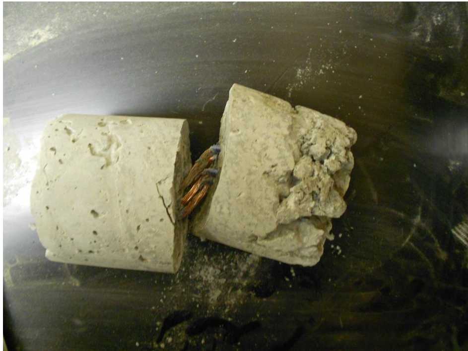
Figure 5.18: Sample H04 Post-test. Two wires were found to be in contact (note that some separation resulted on removing samples from platens).
