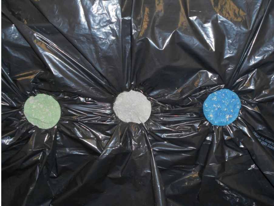
Figure 5.19: Pigmented grout samples in simulated coal face.
