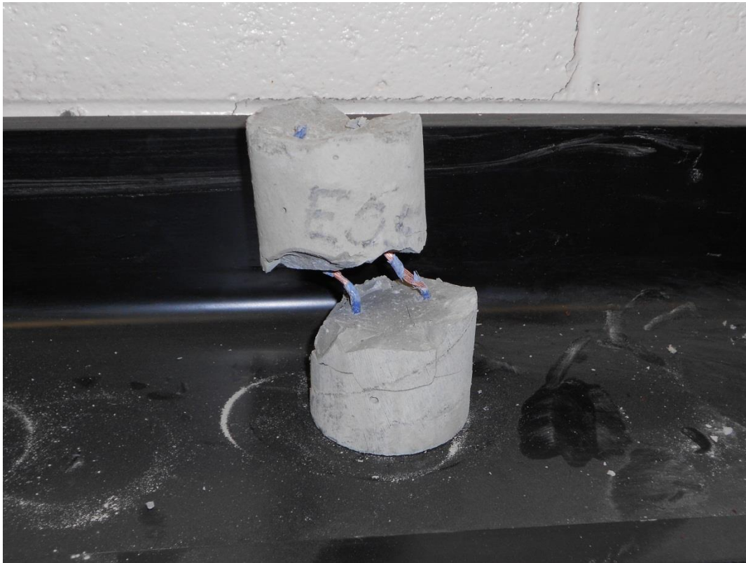
Figure 5.10: Sample E05 Post-Test, after displacement pull.
