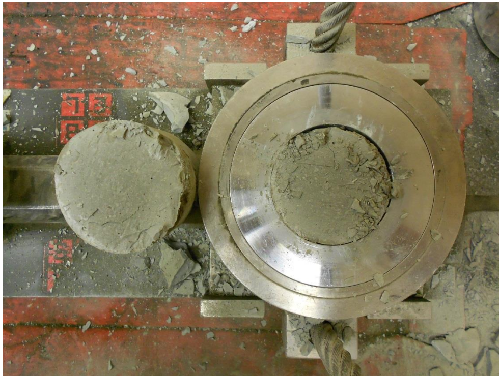
Figure 5.2: Sample A05 Post-Test. Lean grout without embedments.
