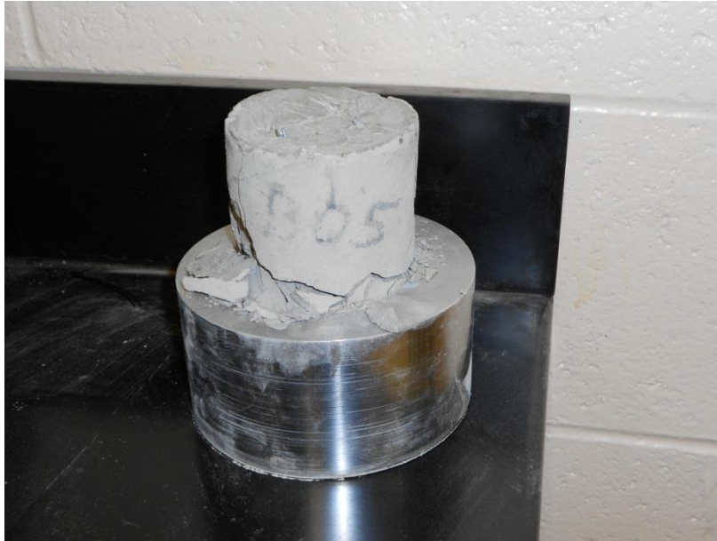
Figure 5.3: Sample B05 Post-Test. Fractures propagating along embedments.
