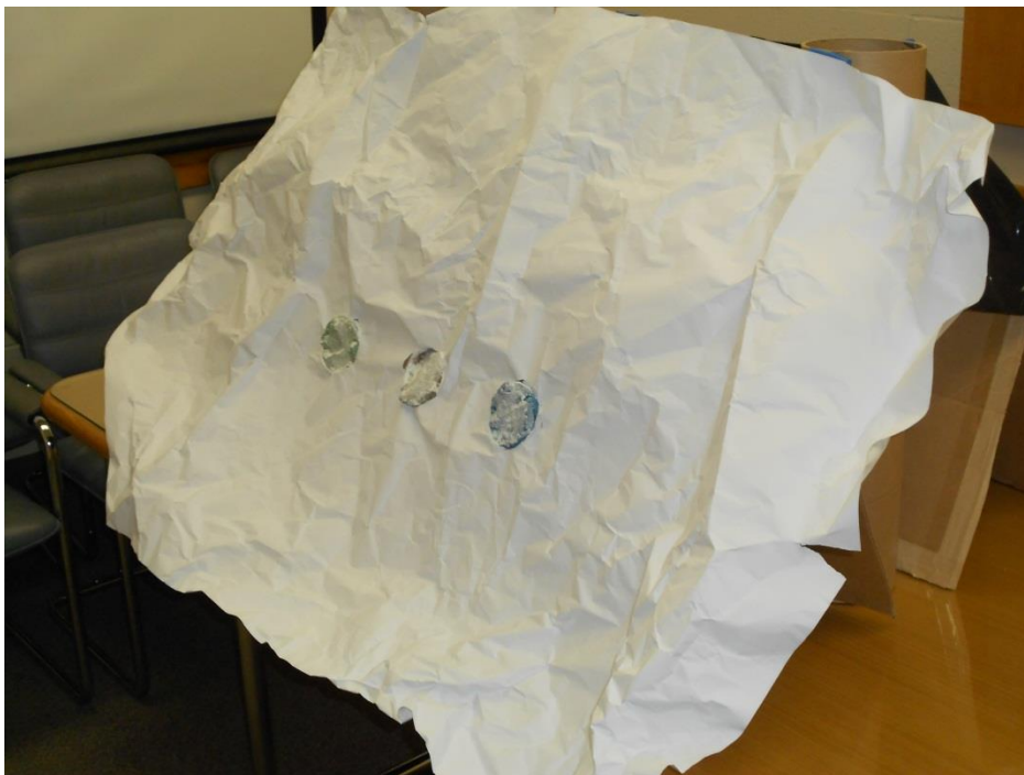
Figure 5.22: Model with light background to simulate coal with rock dust or light-colored rock.
