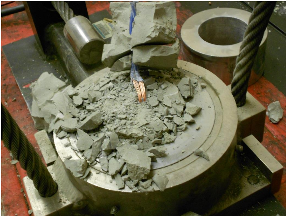
Figure 5.12: Sample F06 Post-Test. On displacement pull, exposed copper wires can make contact.
