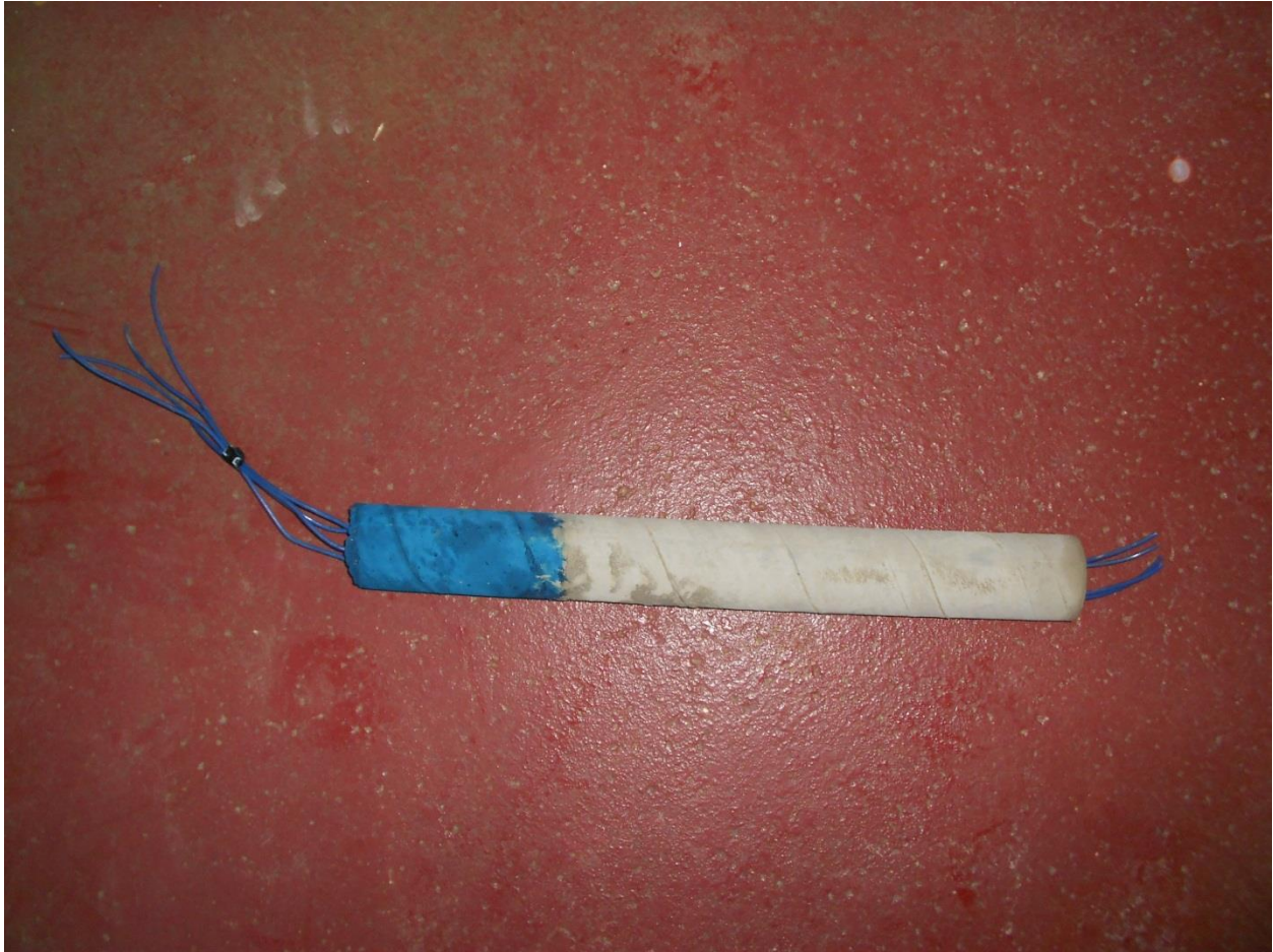
Figure 7.1: 36” Model of Borehole Communication Link with pigmented grout and four conductors.
