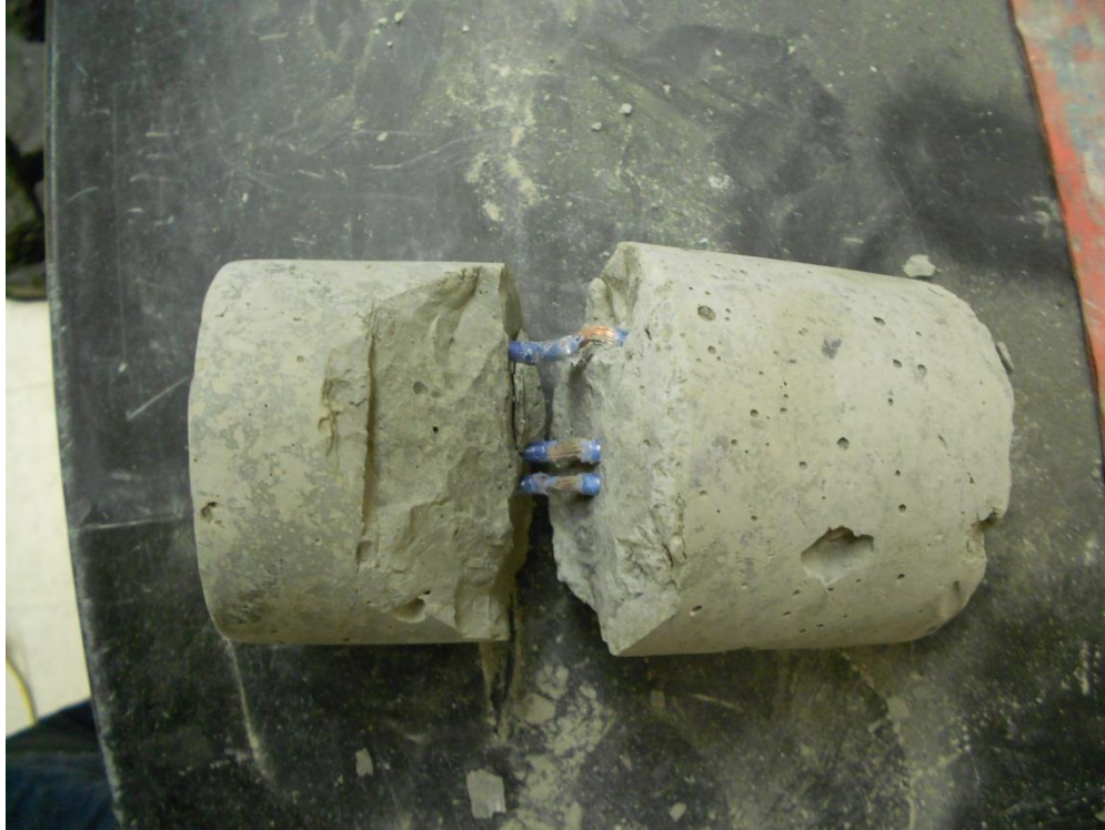
Figure 5.16: Sample J03 Post-test. Note also breakout wedge on left (top of sample).
