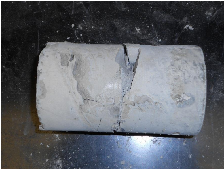
Figure 5.9: Sample E01 Post-Test. Fracture along plane of direct shear load.
