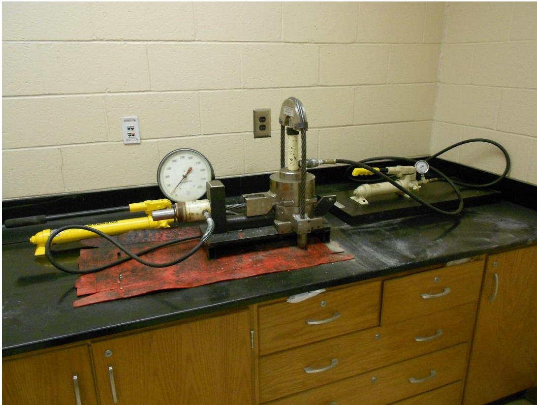
Figure 5.1: Direct shear testing device. Hydraulic press for normal load on top right (white) and for shear load on left (yellow).
