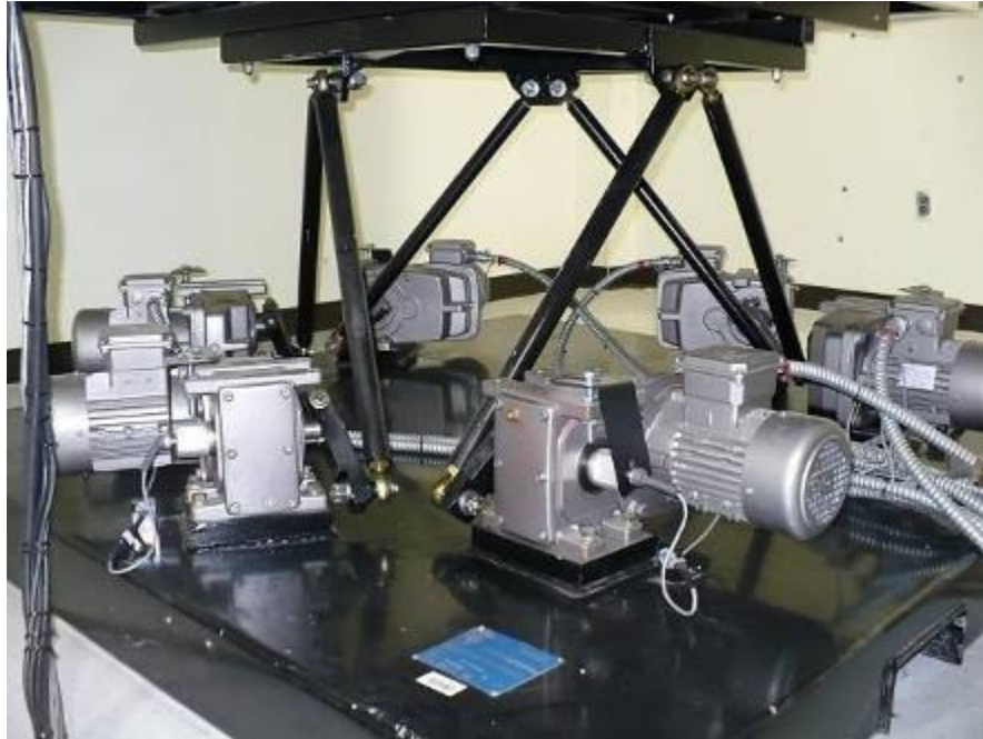
Figure 1-6 Six Electromechanical Actuators for MOTUS Flight Simulator at WVU
