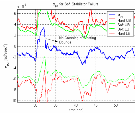
Fig. 5-24-Identification of Soft Stabilator Failure with \omega_{pq}
