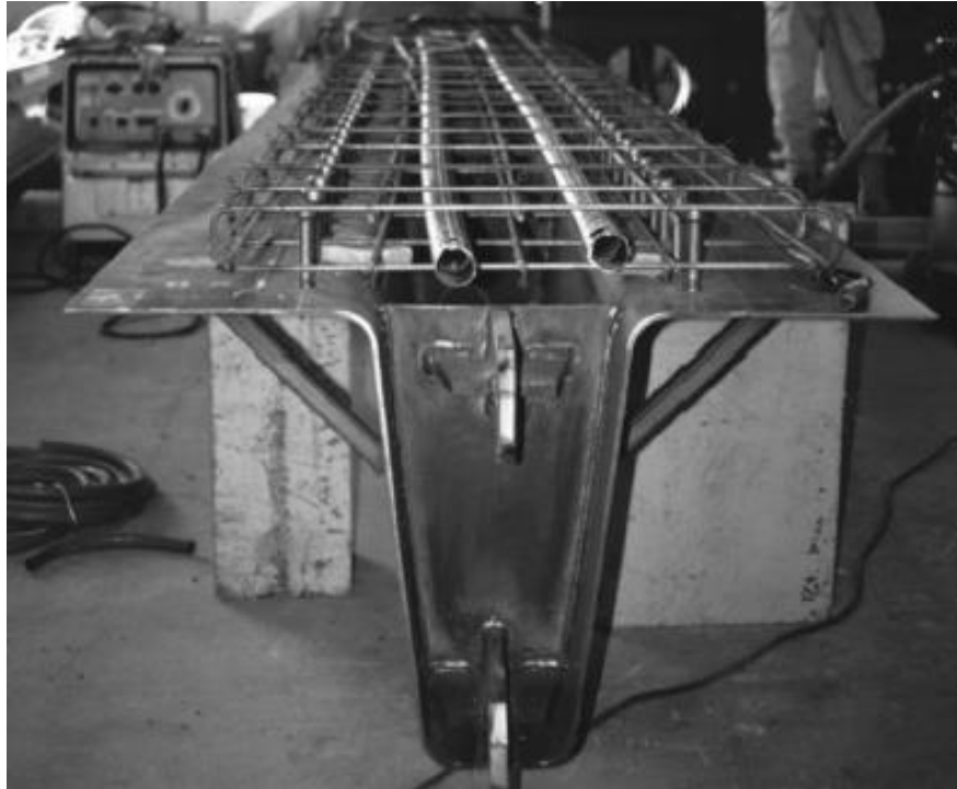
Figure 2.6: Press-Brake-Formed Specimen Proposed by (Nakamura, 2002)
