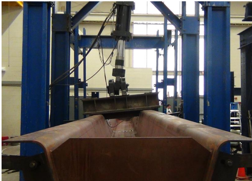
Figure 4.3: Front View of Lateral Torsional Buckling of Specimen #1
