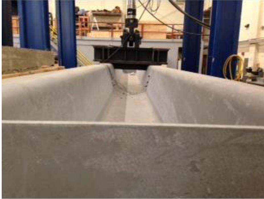
Figure 3.10: Initial Twist of Specimen #2
