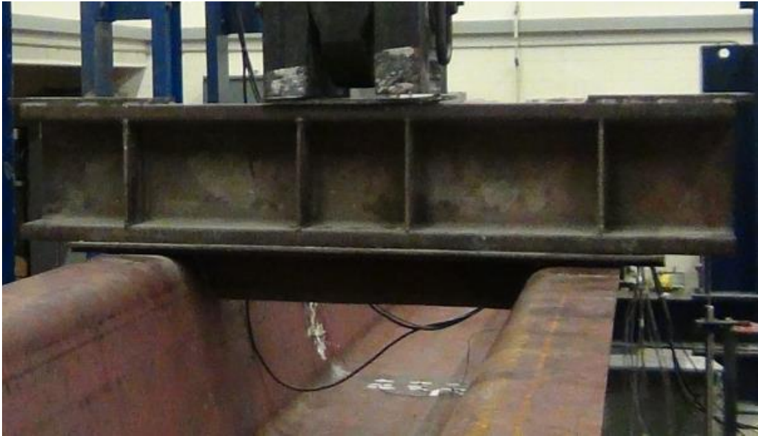
Figure 3.3: Typical Spreader Beam with Elastomeric Pads
