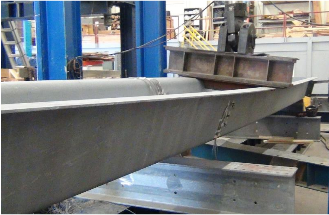
Figure 4.7: Side View of Lateral Torsional Buckling of Specimen #2
