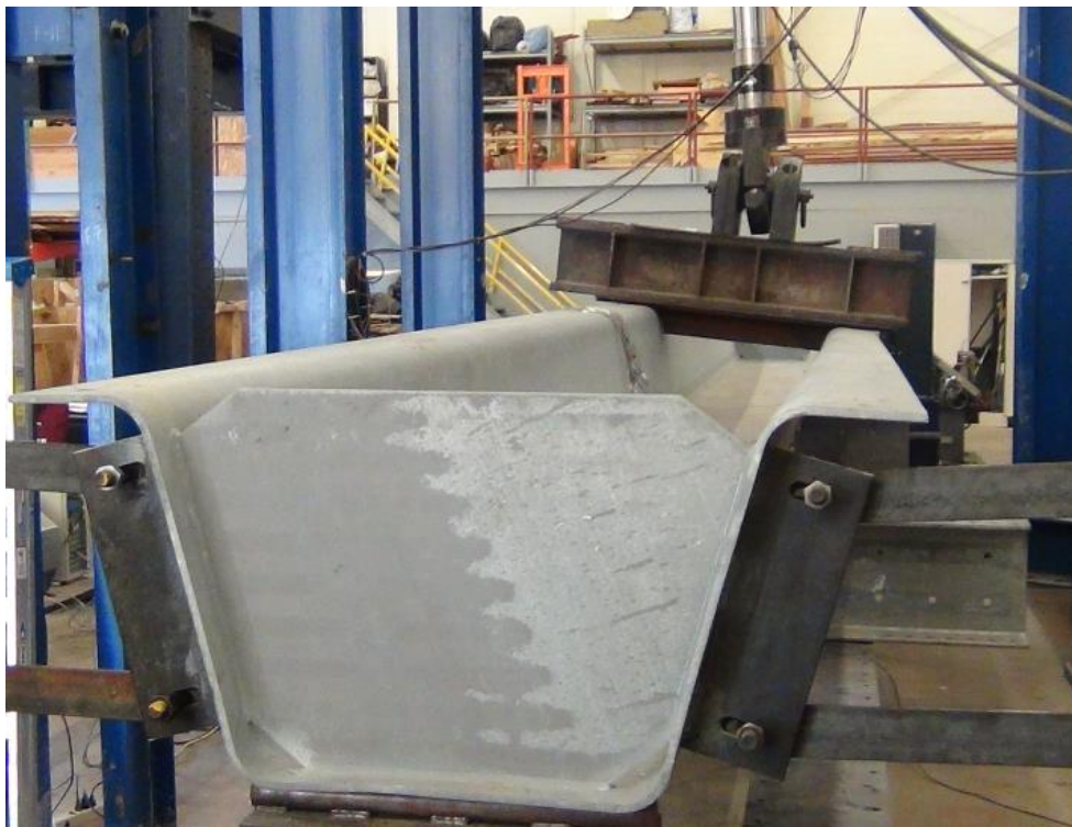
Figure 4.8: Front View of Lateral Torsional Buckling of Specimen #2
